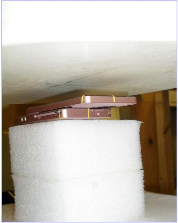
PHT/83567JD04/029: Front of EUT Slide Open Up Antenna Extended Facing Phantom
