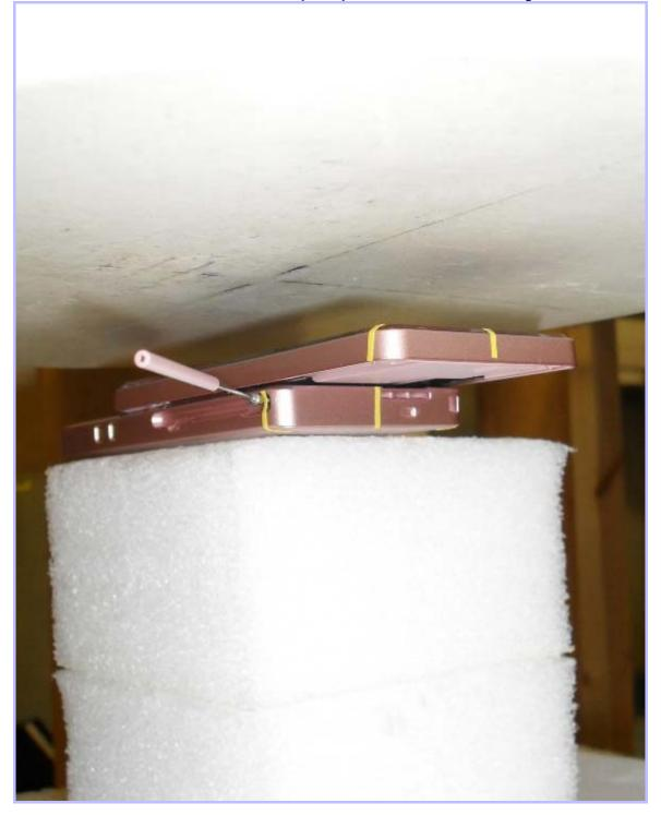
PHT/83567JD04/030: Front of EUT Slide Open Down Antenna Retracted Facing Phantom
