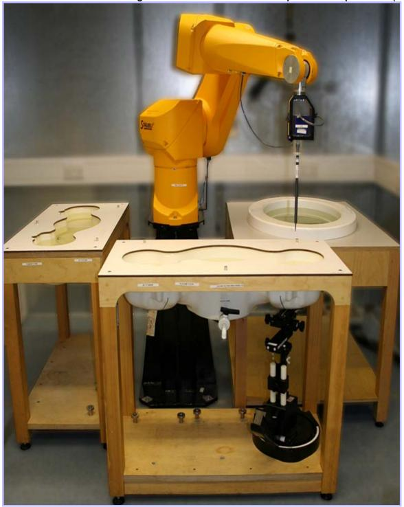
PHT/83567JD04/001: Test configuration for the measurement of Specific Absorption Rate (SAR)
