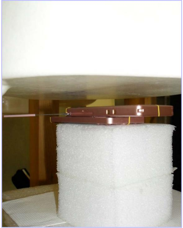
PHT/83567JD04/036: Rear of EUT Slide Open Down Antenna Retracted Facing Phantom
