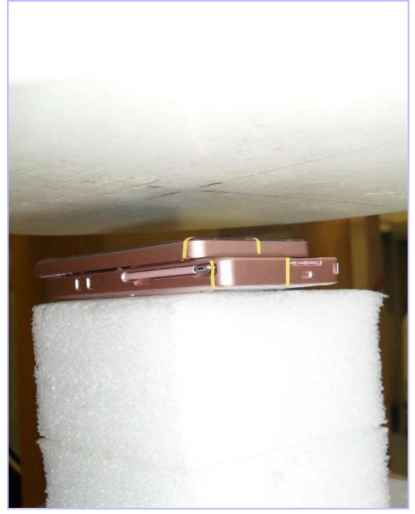
PHT/83567JD04/031: Front of EUT Slide Open Down Antenna Extended Facing Phantom
