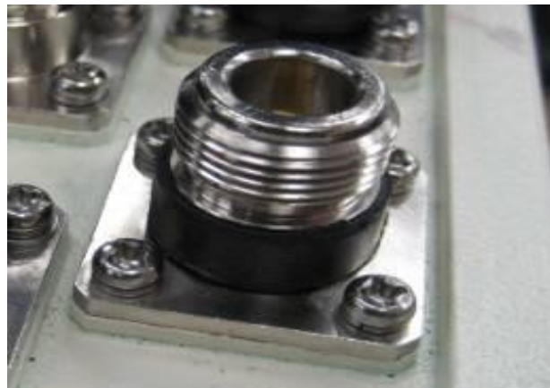
Figure 28. Butyl Rubber Ring Finished
