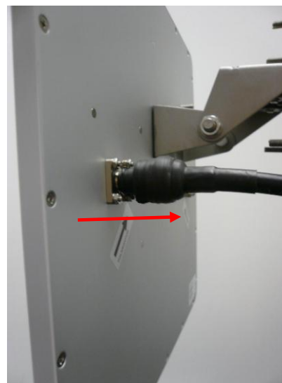
Figure 24. Waterproof wrapping direction
