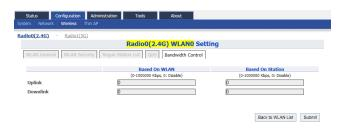
Figure 72 – Bandwidth Control Setting on WLAN 0-15
