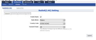
Figure 32 – Radio0 General Setting of Station
