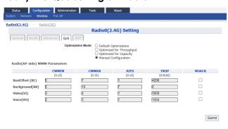
Figure 70 – QoS Setting on Radio
