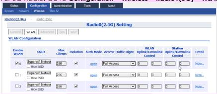
Figure 9 - Radio 2.4G WLAN List
