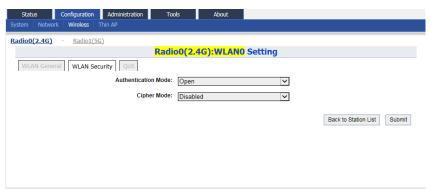
Figure 35 – Security Setting of Station
