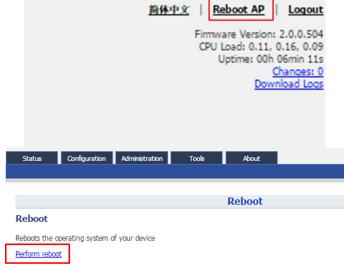
Figure 6 - Reboot the device via Web UI
