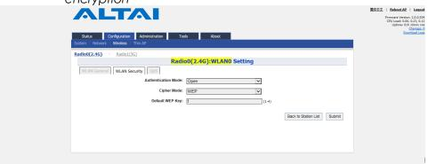
Figure 36 – Open network with WEP of Station
