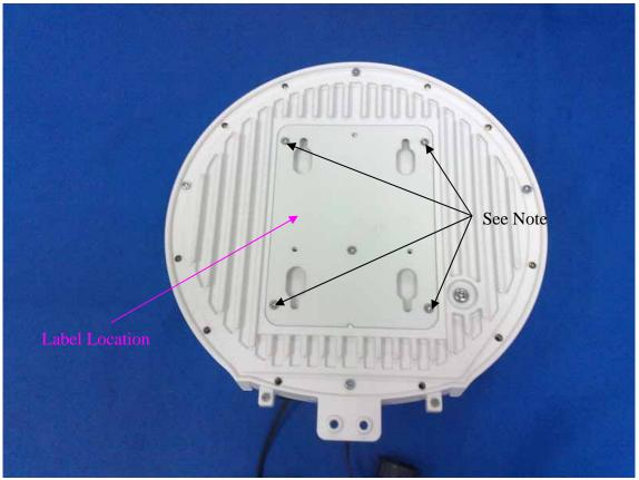
Note: This four screws will be applied strong adhesive glue and cannot be removed. And the label is also not easy to wear off, as there is heat sink (edges) in the surrounding.
