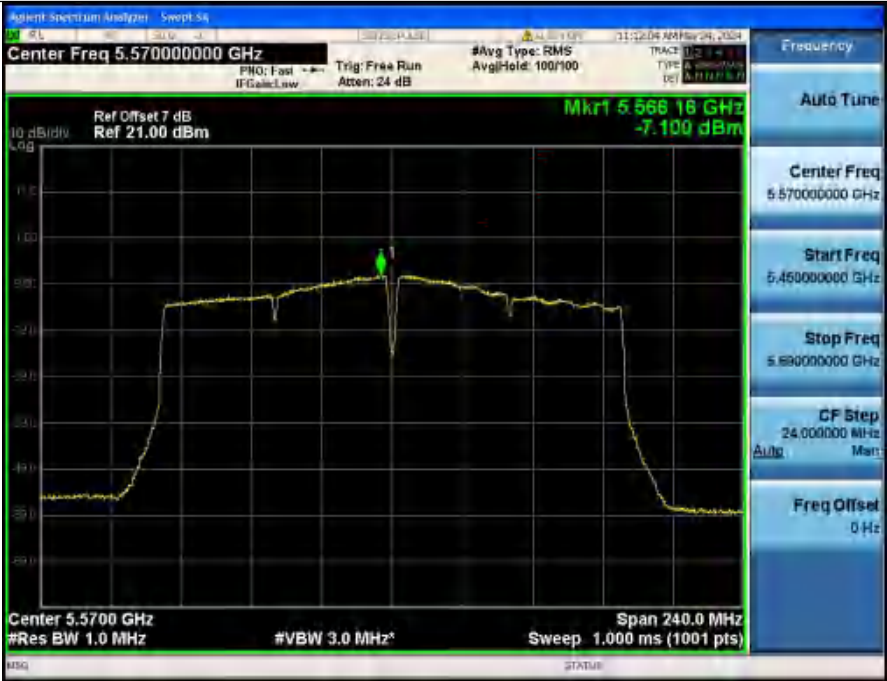
Power Spectral Density NVNT ANT2 802_11ac(VHT160) 5570
