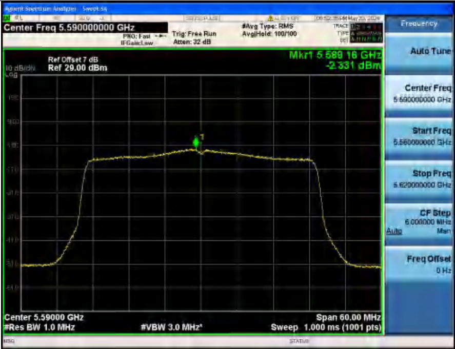
Power Spectral Density NVNT_ANT2_802_11ax(HE40)_5590
