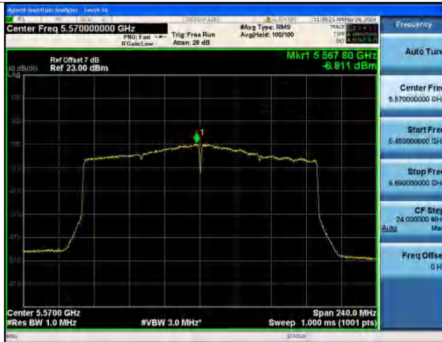
Power Spectral Density NVNT ANT2 802.11ax(HE160) 5570
