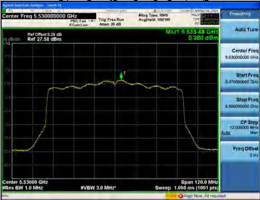
Power Spectral Density NVNT_ANT2_802_11ax(HE80)_5530
