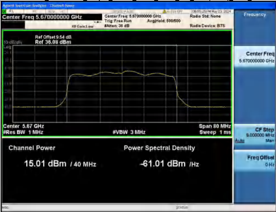
Maximum Conducted Output Power NVNT ANT2_802_11ax(HE40) 5670_40M
