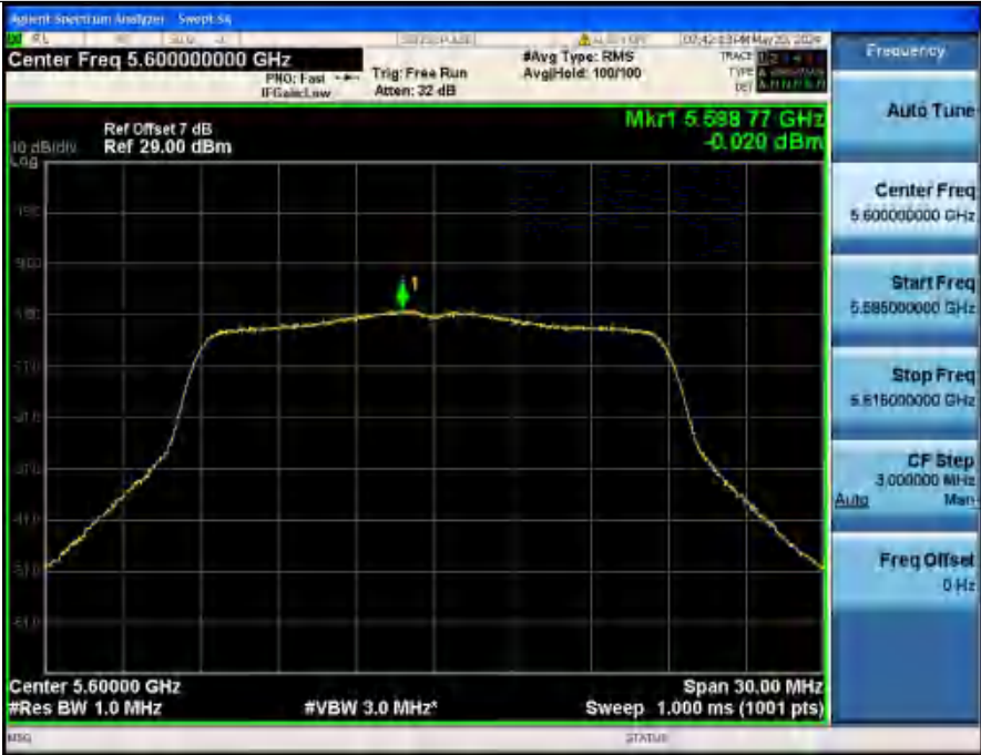
Power Spectral Density NVNT ANT2_802_11n(HT20)_5600
