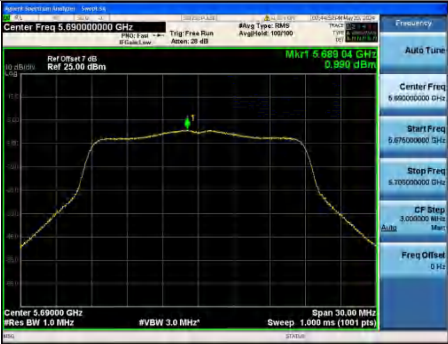
Power Spectral Density NVNT ANT2_802_11n(HT20)_5700
