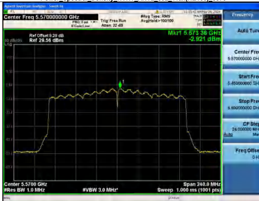
Power Spectral Density NVNT ANT2 802.11ax(HE160) 5570
