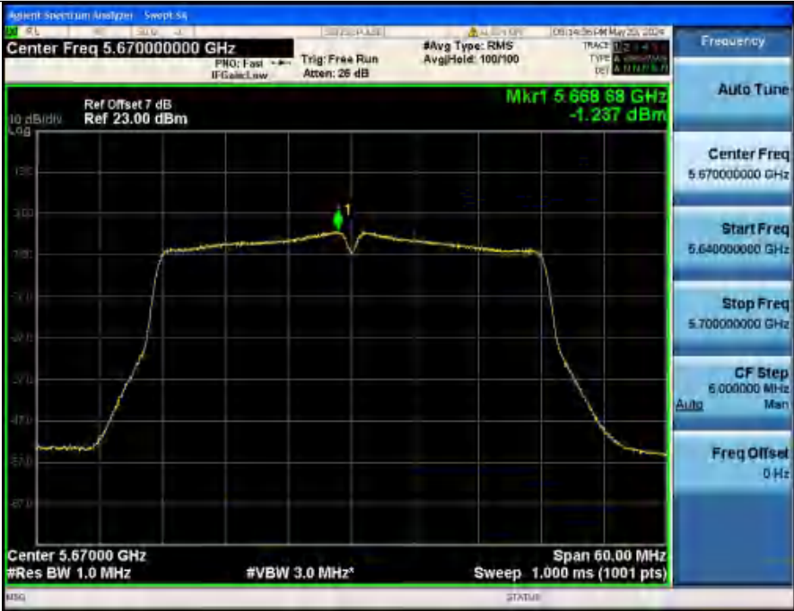
Power Spectral Density NVNT ANT2_802_11n(HT40)_5670
