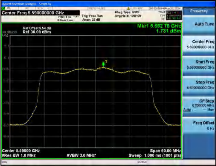
Power Spectral Density NVNT_ANT2_802_11ax(HE40)_5590
