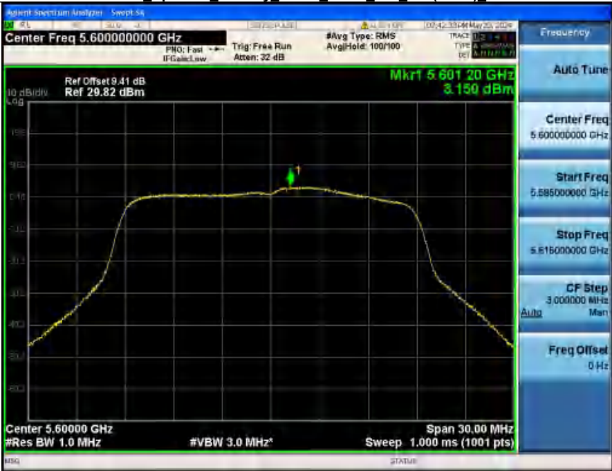
Power Spectral Density NVNT ANT2_802_11n(HT20)_5600
