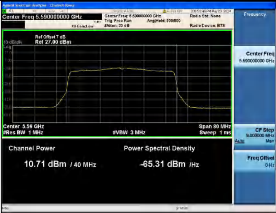
Maximum Conducted Output Power NVNT ANT2_802_11ax(HE40) 5590 40M
