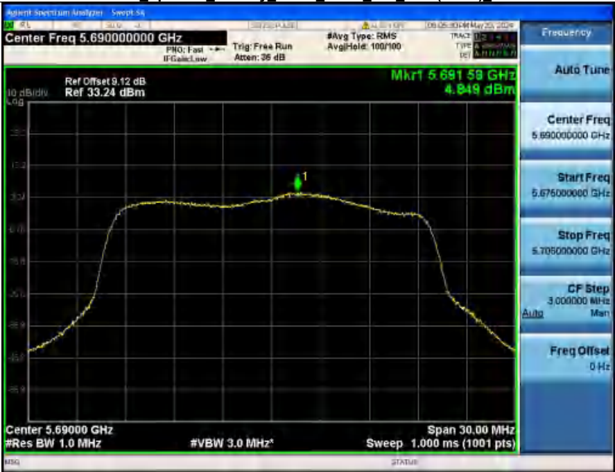
Power Spectral Density NVNT_ANT2_802_11ax(HE20)_5700
