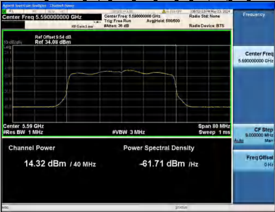
Maximum Conducted Output Power NVNT ANT2_802_11ax(HE40) 5590 40M
