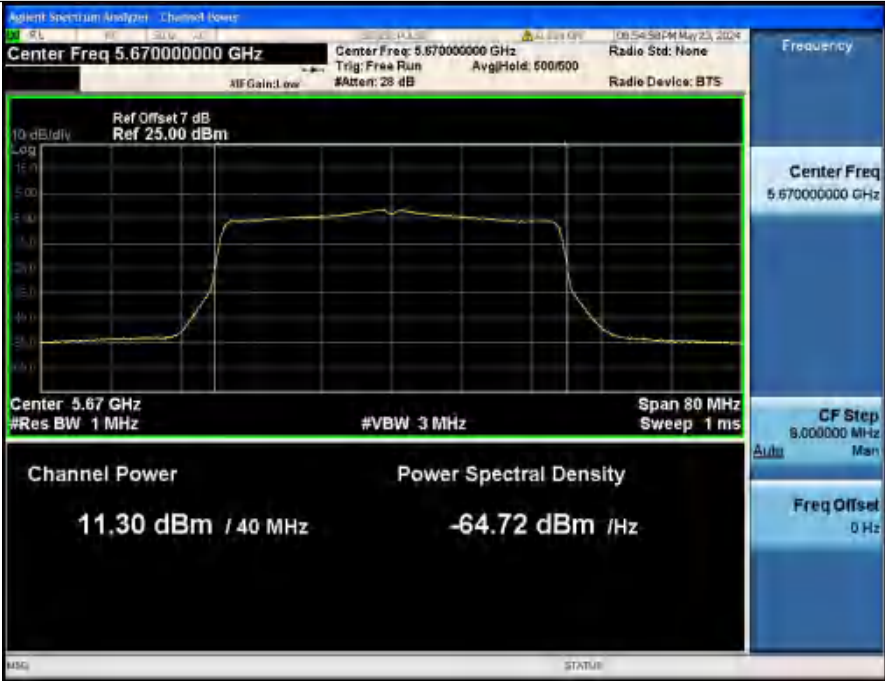
Maximum Conducted Output Power NVNT ANT2_802_11ax(HE40) 5670_40M
