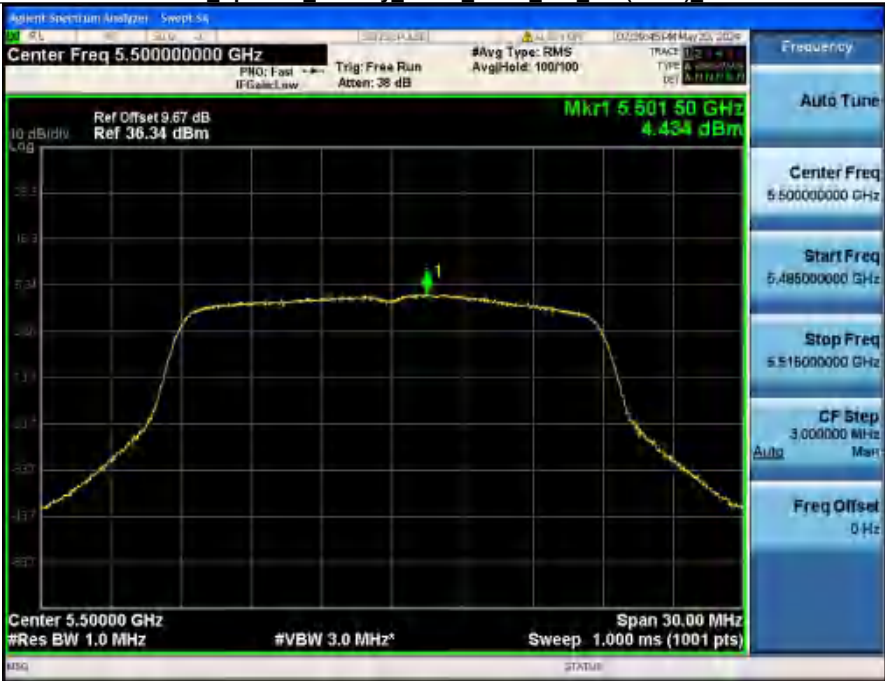
Power Spectral Density NVNT ANT2_802_11n(HT20)_5500
