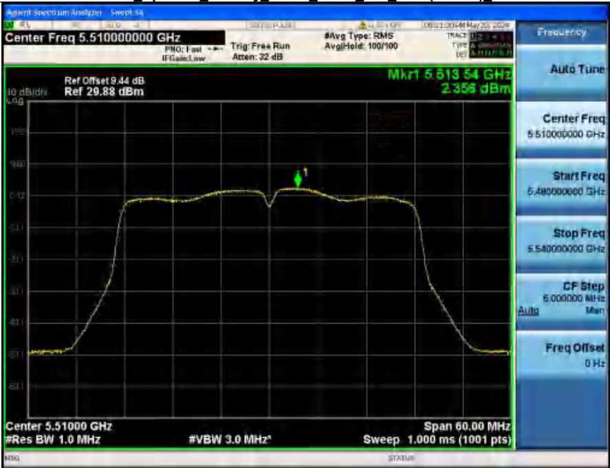
Power Spectral Density NVNT_ANT2_802_11ac(VHT40)_5510
