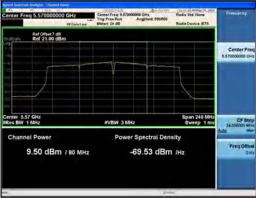
Maximum Conducted Output Power_NVNT ANT2_802_11ac(VHT160)_5570_160M
