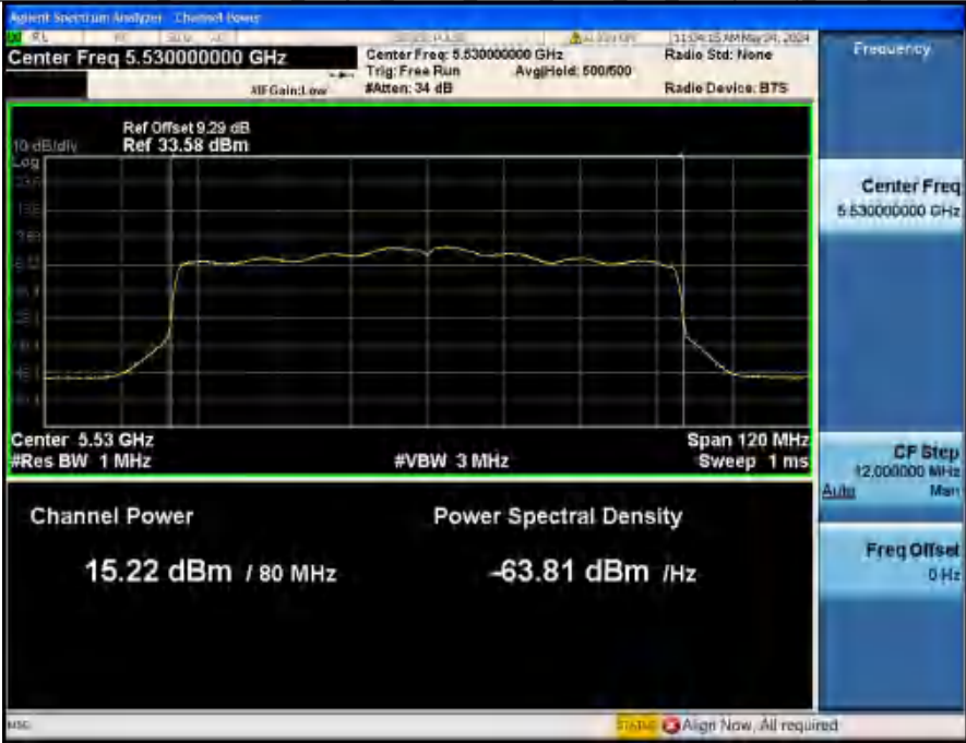
Maximum Conducted Output Power NVNT ANT2_802_11ax(HE80)_5530_80M
