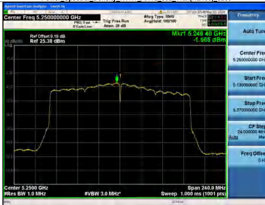
Power Spectral Density NVNT ANT2 802.11ax(HE160) 5250
