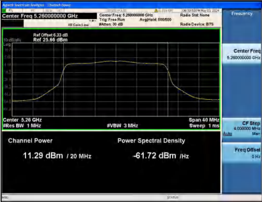
Maximum Conducted Output Power NVNT ANT2_802_11ax(HE20)_5260_20M
