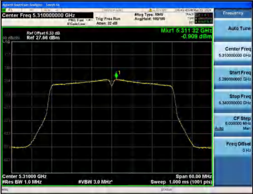
Power Spectral Density NVNT ANT2_802_11n(HT40)_5310
