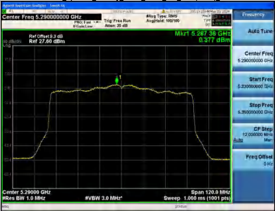
Power Spectral Density NVNT_ANT2_802_11ax(HE80)_5290
