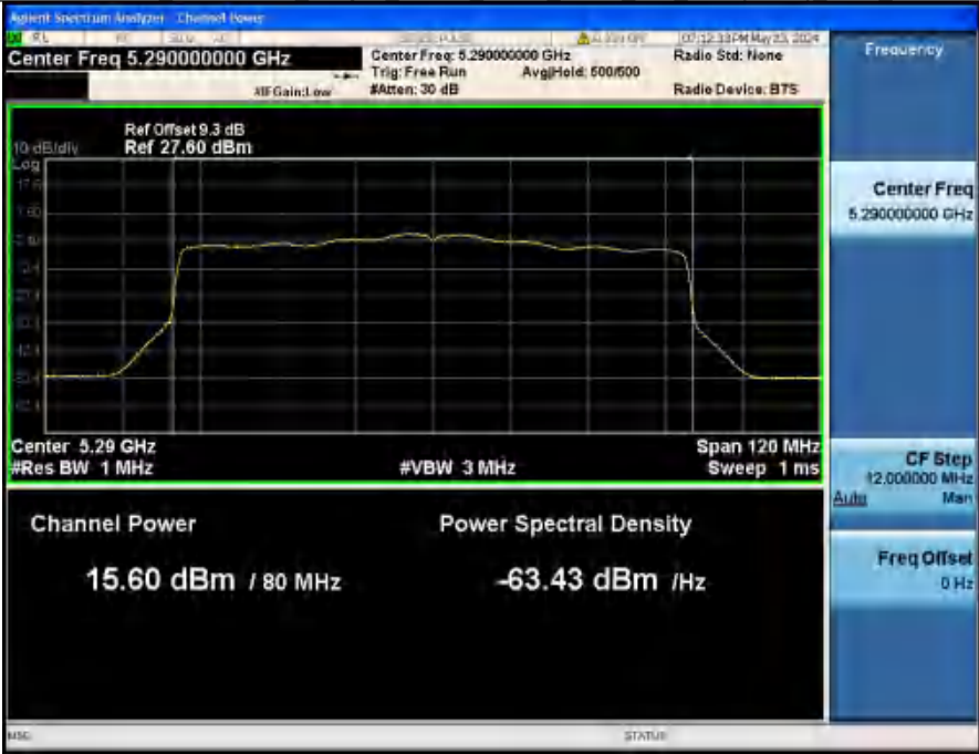
Maximum Conducted Output Power NVNT ANT2_802_11ax(HE80)_5290_80M
