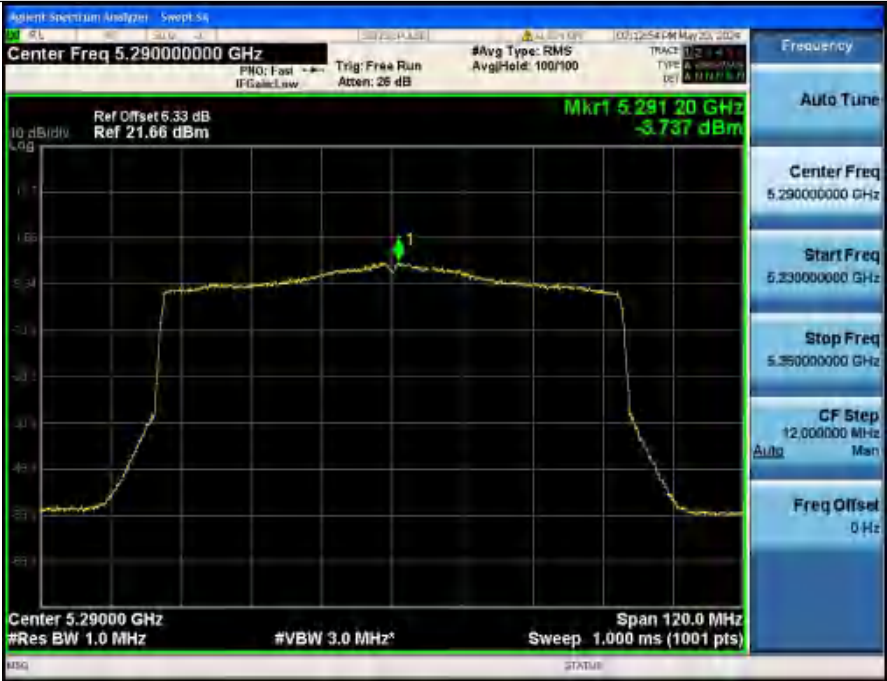
Power Spectral Density NVNT_ANT2_802_11ax(HE80)_5290
