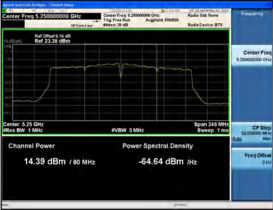
Maximum Conducted Output Power NVNT ANT2 802 11ac(VHT160) 5250 160M
