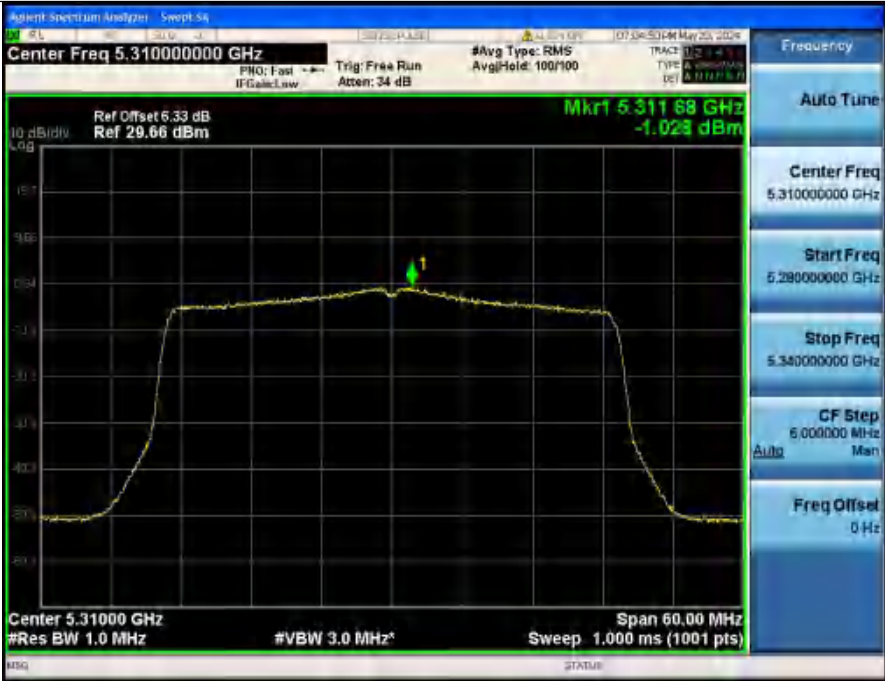
Power Spectral Density NVNT_ANT2_802_11ax(HE40)_5310
