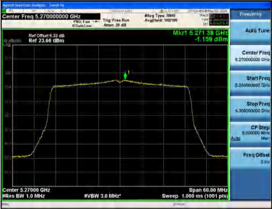
Power Spectral Density NVNT_ANT2_802_11ax(HE40)_5270
