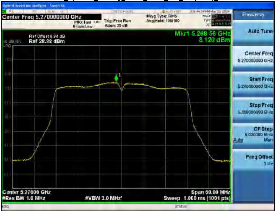
Power Spectral Density NVNT ANT2_802_11n(HT40)_5270
