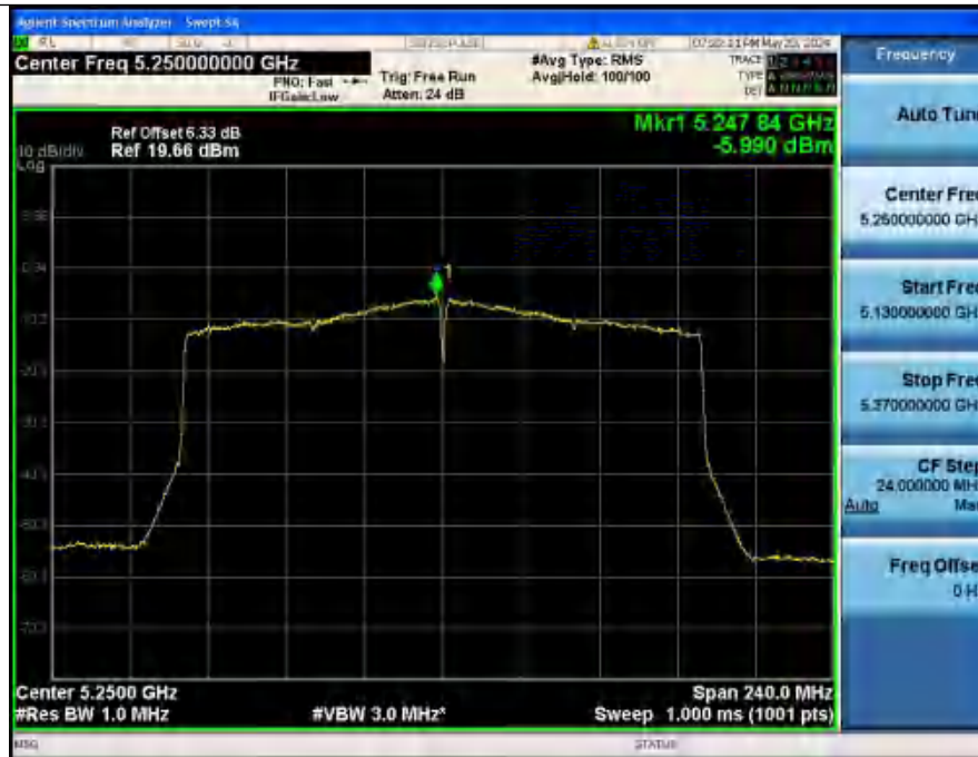
Power Spectral Density NVNT ANT2 802.11ax(HE160) 5250
