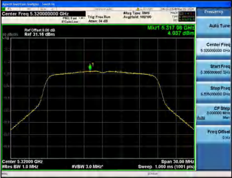
Power Spectral Density NVNT ANT2_802_11n(HT20)_5320
