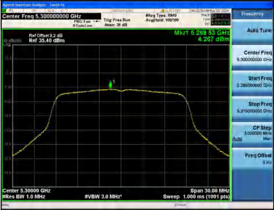
Power Spectral Density NVNT ANT2_802_11n(HT20)_5300
