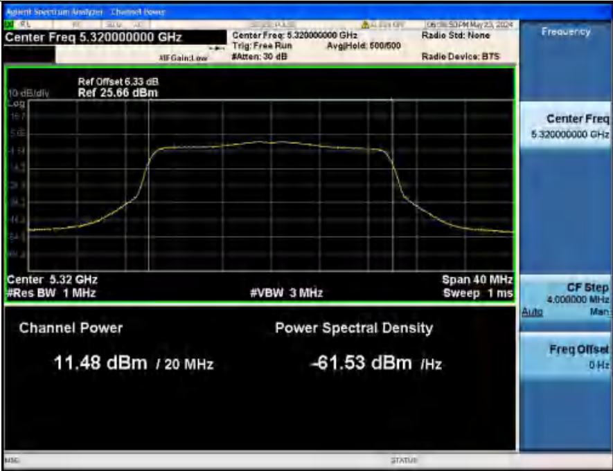
Maximum Conducted Output Power NVNT_ANT2_802_11ax(HE20)_5320_20M
