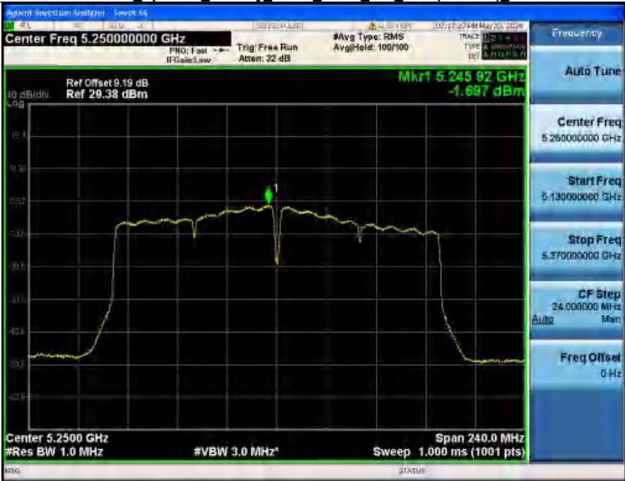
Power Spectral Density NVNT ANT2 802_11ac(VHT160) 5250
