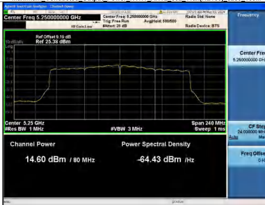
Maximum Conducted Output Power NVNT ANT2_802_11ax(HE160) 5250 160M
