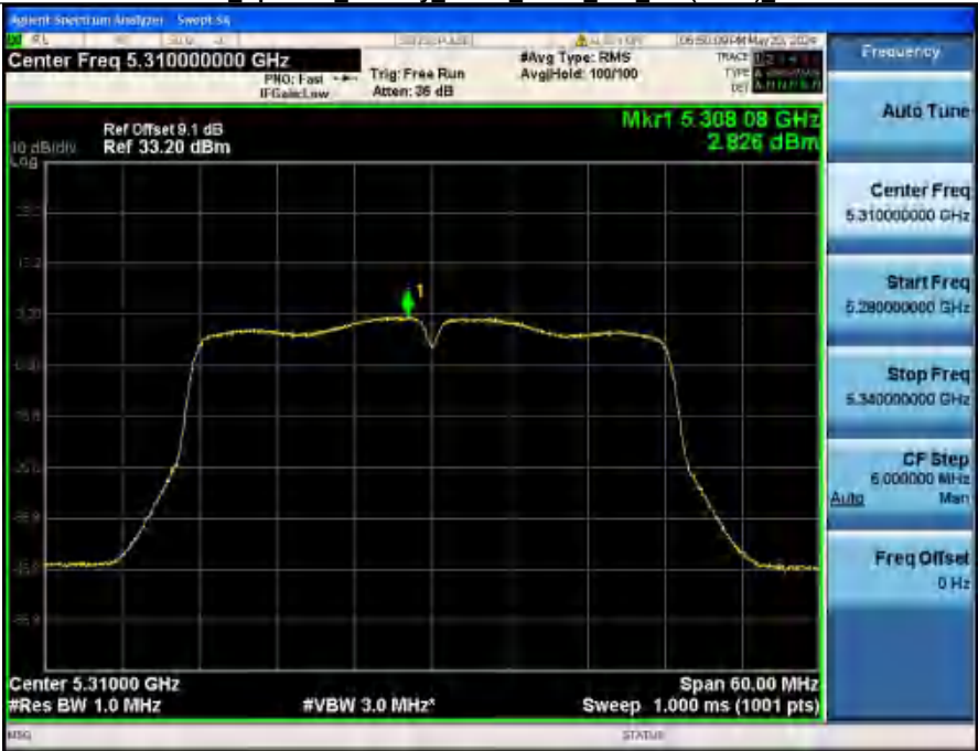
Power Spectral Density NVNT ANT2_802_11n(HT40)_5310
