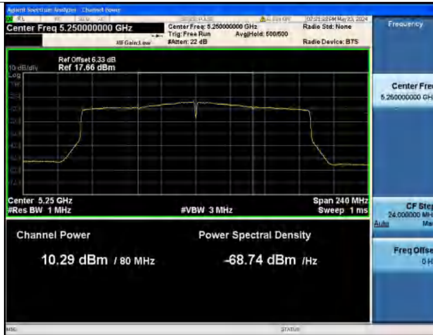
Maximum Conducted Output Power NVNT ANT2_802_11ax(HE160) 5250 160M
