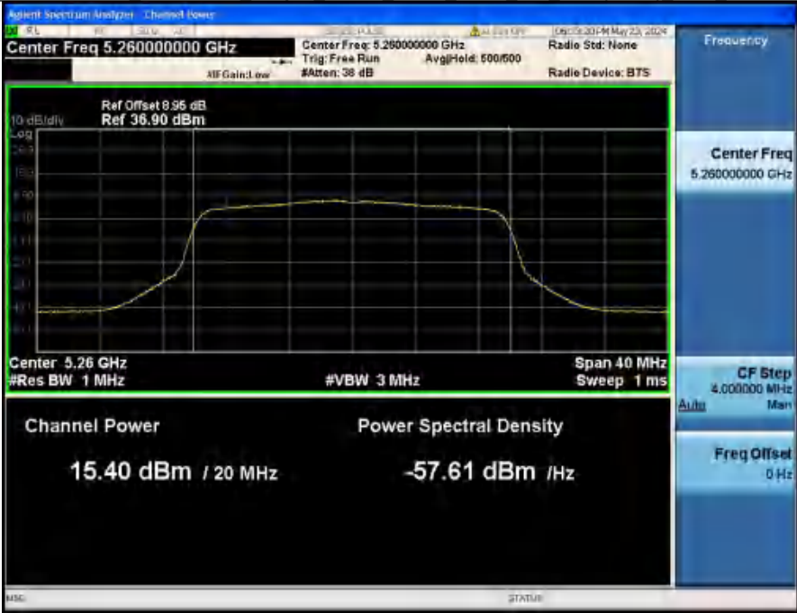
Maximum Conducted Output Power NVNT ANT2_802_11ax(HE20)_5260_20M
