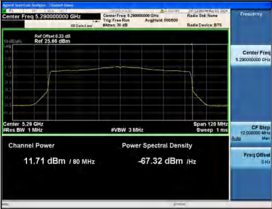
Maximum Conducted Output Power NVNT ANT2_802_11ax(HE80)_5290_80M
