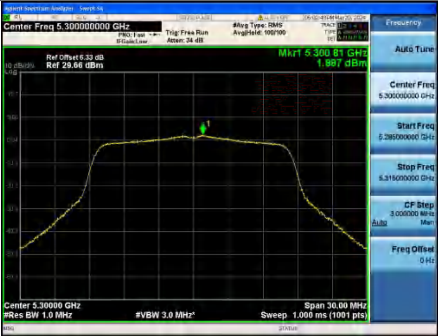
Power Spectral Density_NVNT_ANT2_802_11a_5300
