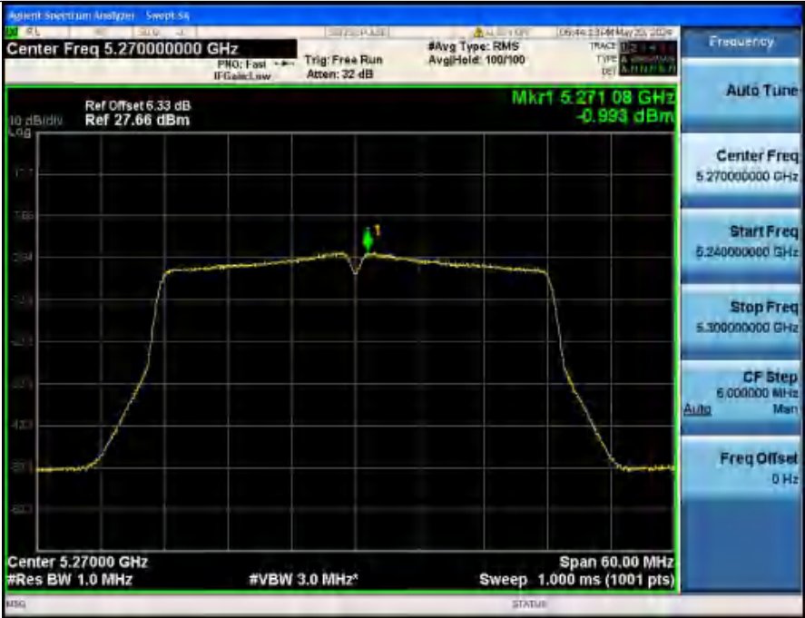
Power Spectral Density NVNT ANT2_802_11n(HT40)_5270
