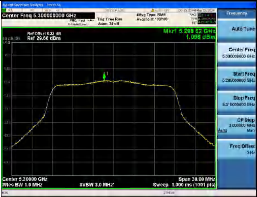
Power Spectral Density NVNT ANT2_802_11n(HT20)_5300
