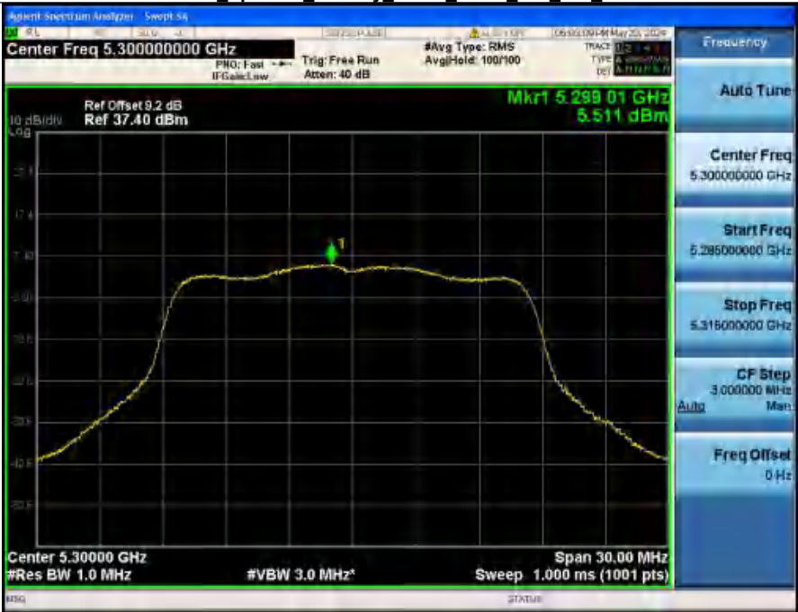
Power Spectral Density_NVNT_ANT2_802_11a_5300
