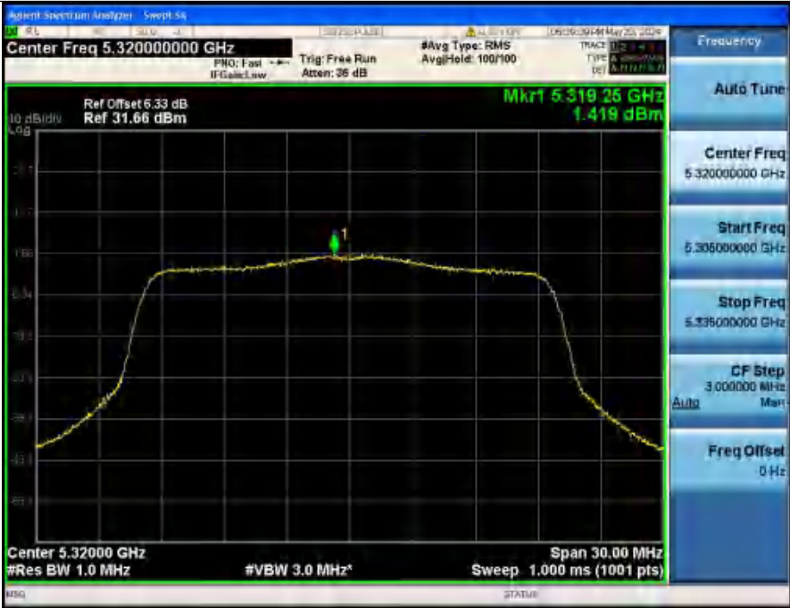
Power Spectral Density NVNT_ANT2_802_11ax(HE20)_5320
