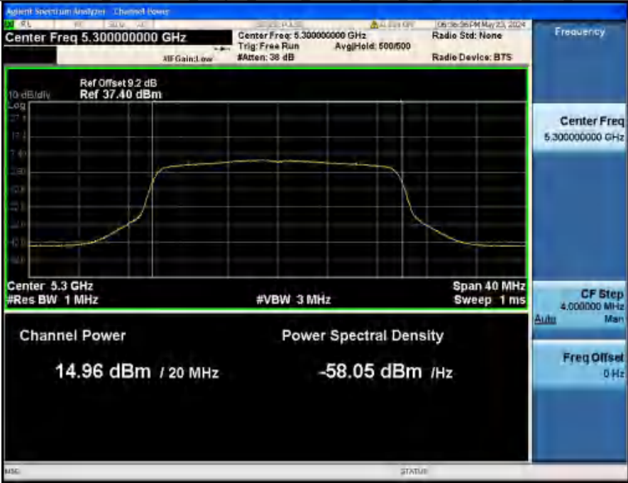
Maximum Conducted Output Power NVNT_ANT2_802_11ax(HE20)_5300_20M
