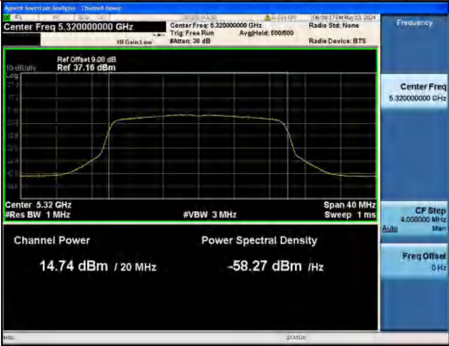
Maximum Conducted Output Power NVNT_ANT2_802_11ax(HE20)_5320_20M
