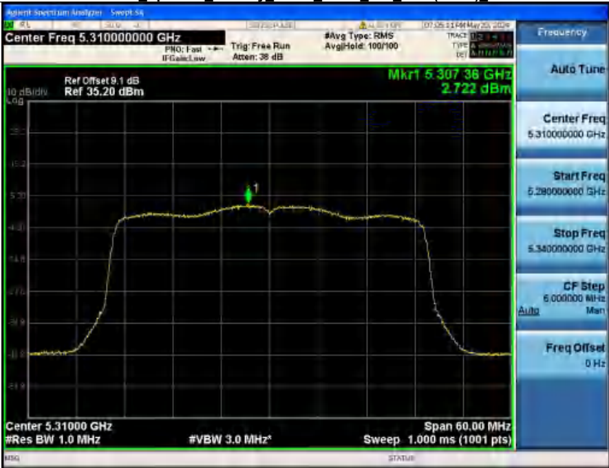
Power Spectral Density NVNT_ANT2_802_11ax(HE40)_5310
