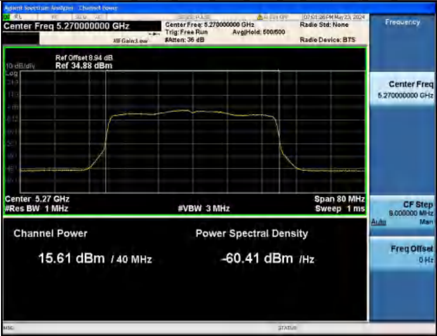
Maximum Conducted Output Power NVNT ANT2_802_11ax(HE40)_5270_40M
