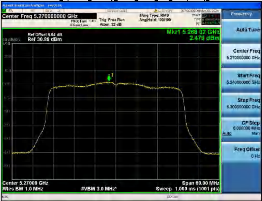
Power Spectral Density NVNT_ANT2_802_11ax(HE40)_5270
