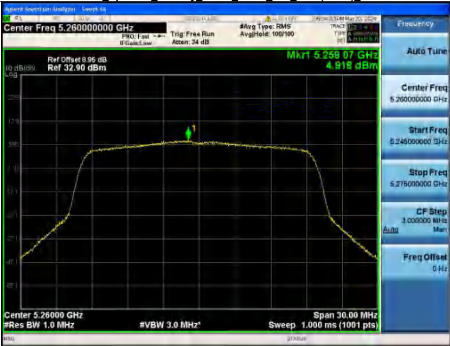
Power Spectral Density NVNT_ANT2_802_11ax(HE20)_5260
