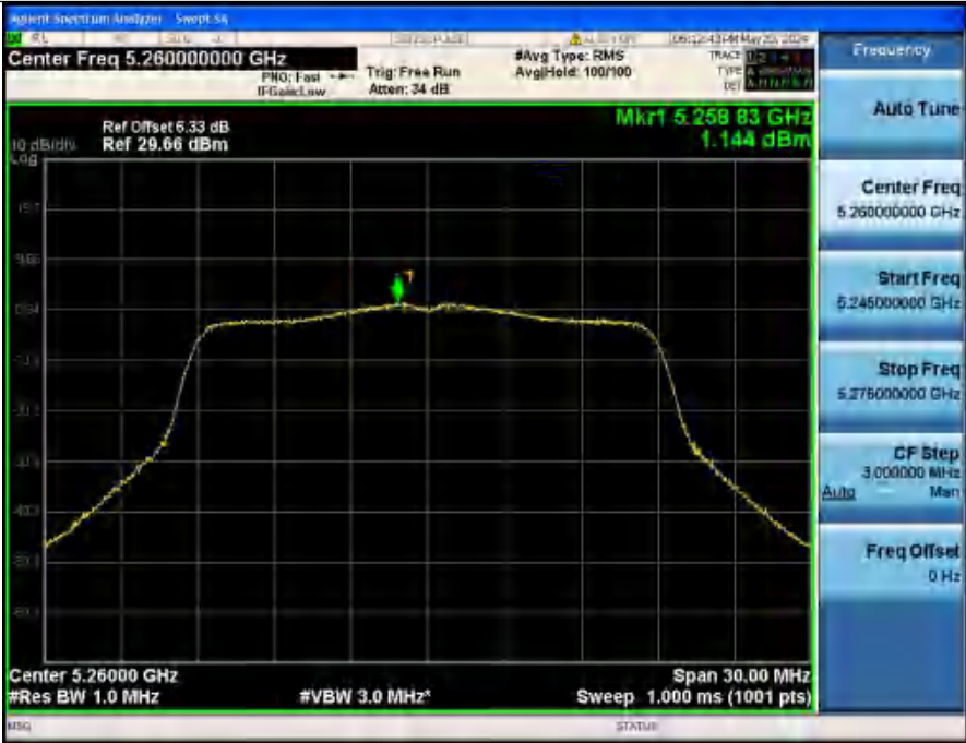
Power Spectral Density NVNT ANT2_802_11n(HT20)_5260
