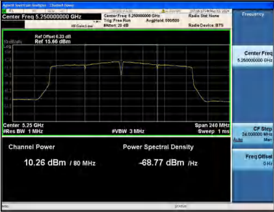
Maximum Conducted Output Power NVNT ANT2 802 11ac(VHT160) 5250 160M
