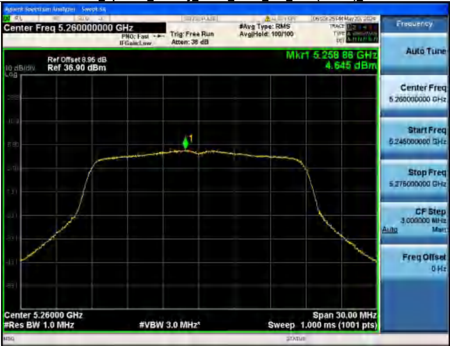
Power Spectral Density_NVNT_ANT2_802_11ac(VHT20)_5260
