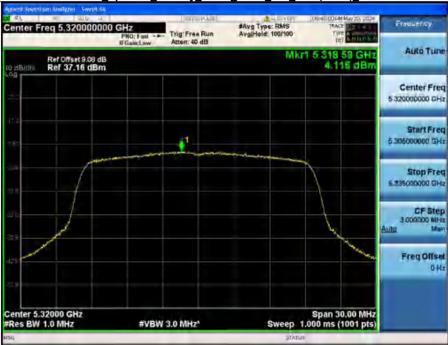
Power Spectral Density NVNT_ANT2_802_11ax(HE20)_5320
