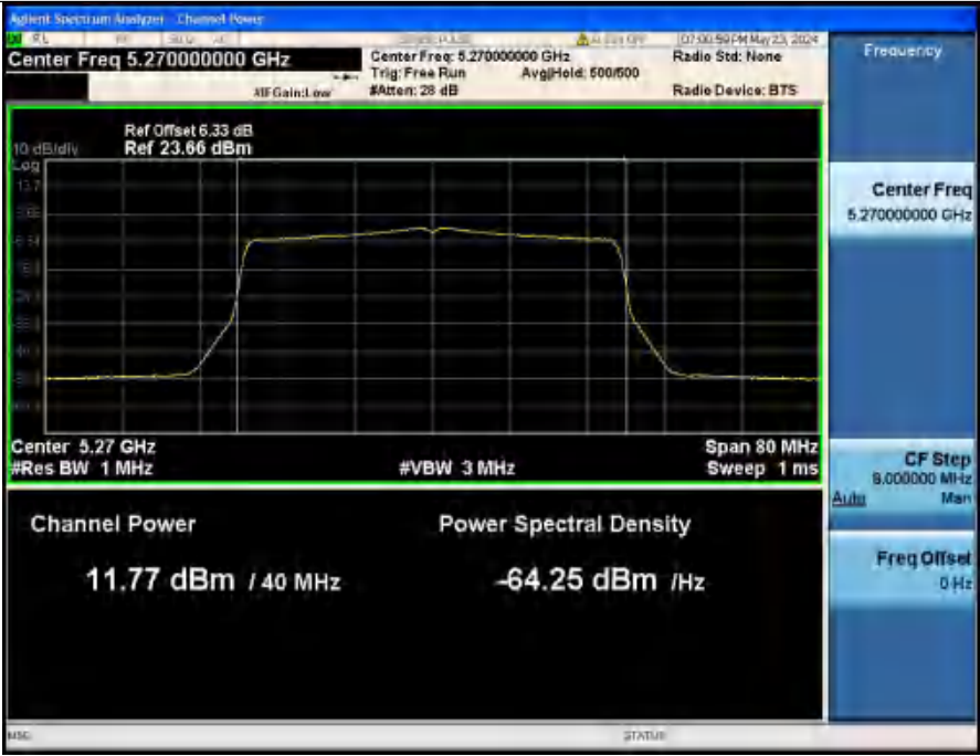
Maximum Conducted Output Power NVNT ANT2_802_11ax(HE40)_5270_40M
