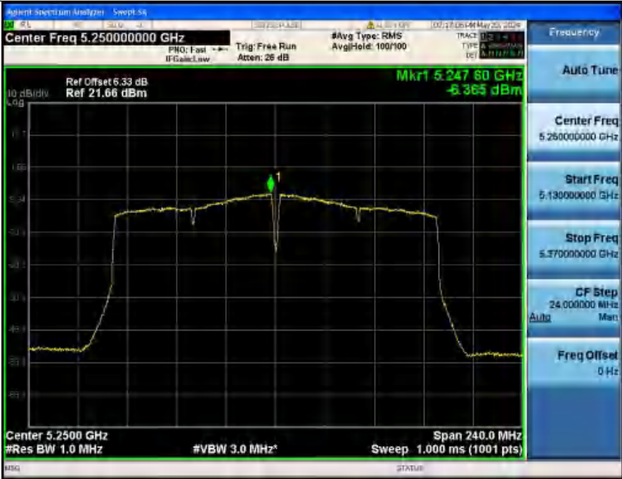
Power Spectral Density NVNT ANT2 802_11ac(VHT160) 5250
