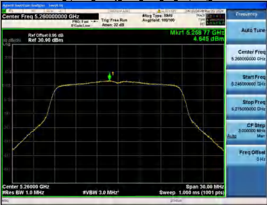
Power Spectral Density NVNT ANT2_802_11n(HT20)_5260
