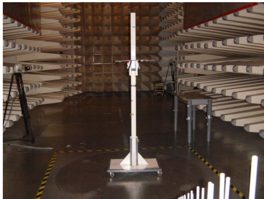
Set-up for Radiated Emission Test
