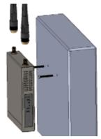
Step 2. Connect omni antennas (item C in the 错误! 未找到引用源。), power cord, PoE (item D and E in the 错误! 未找到引用源。), and Ethernet cables to the APC:
