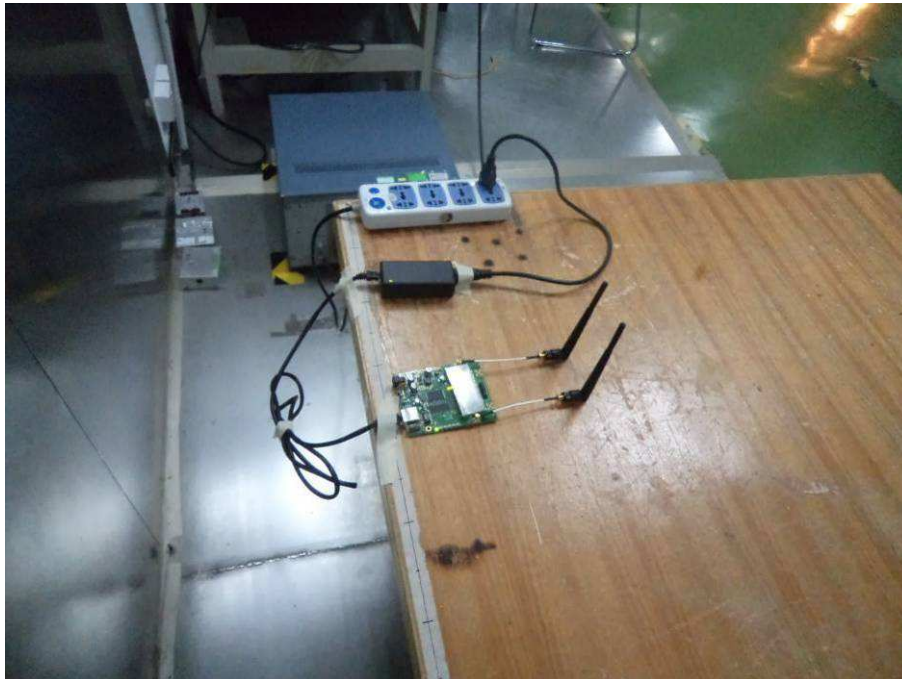
Conducted Emissions- Side View (PoE Power)
