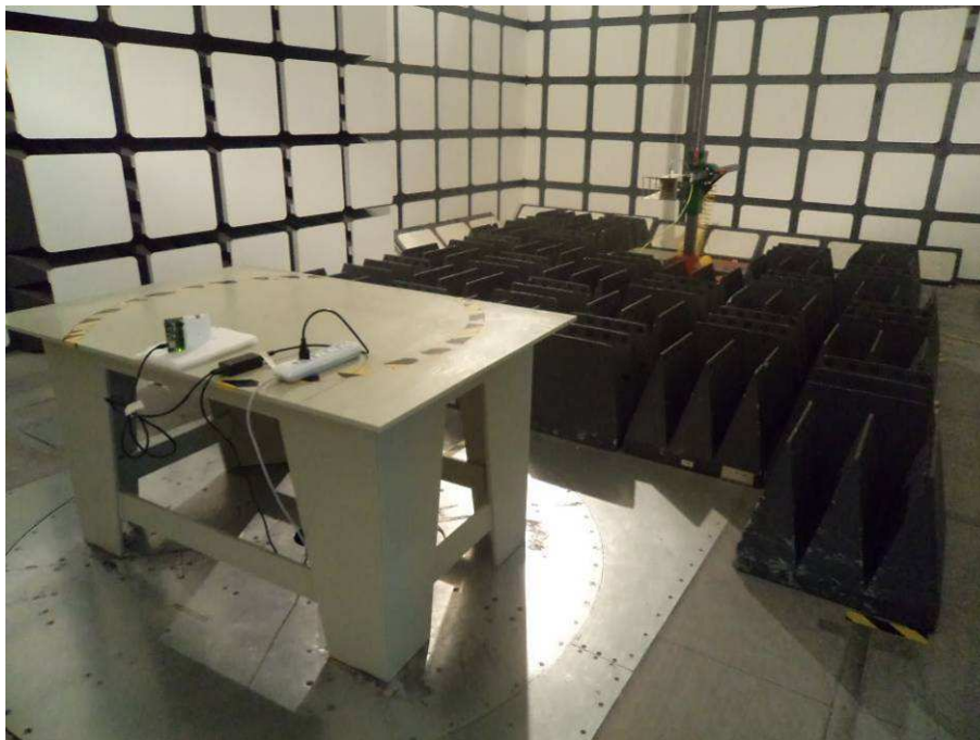
Radiated Emissions View (Above 1 GHz, 8dBi Antenna)
