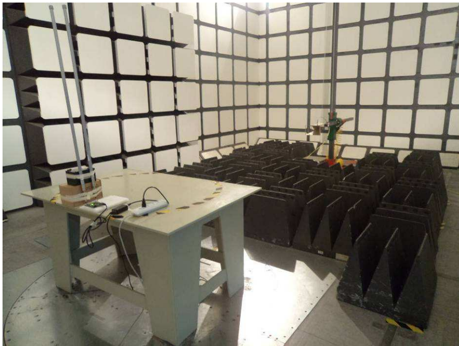
Radiated Emissions View (Above 1 GHz, 12dBi Antenna)
