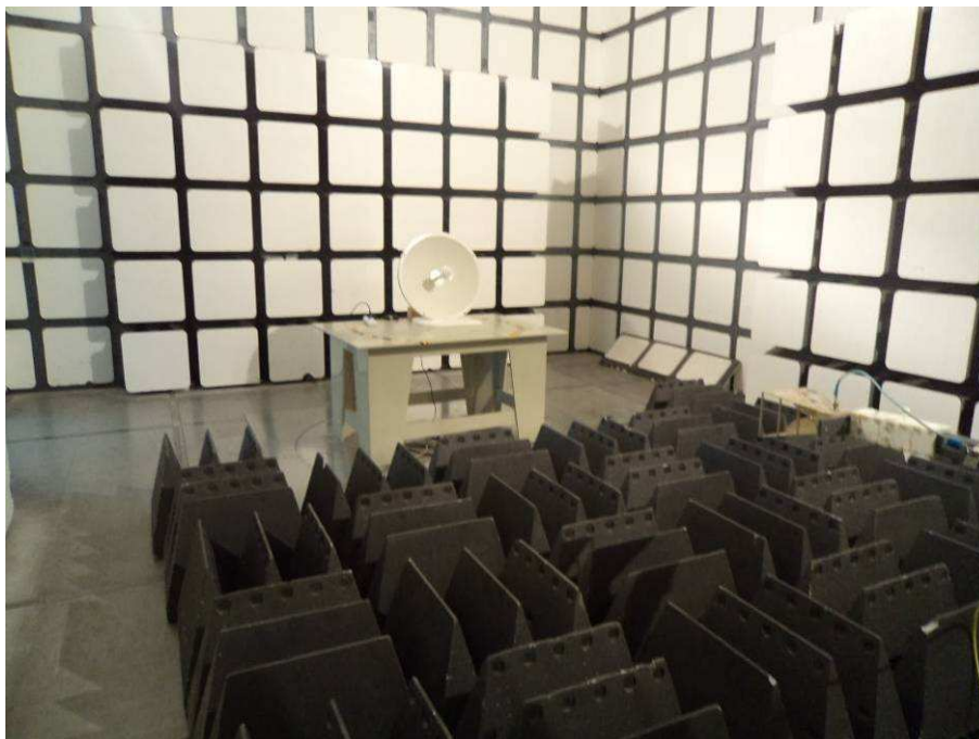
Radiated Emissions View (Above 1 GHz, 24dBi Antenna)
