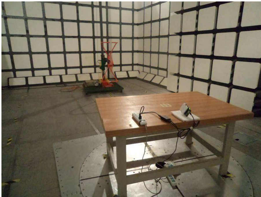
Radiated Emissions View (Below 1 GHz, 8dBi Antenna)
