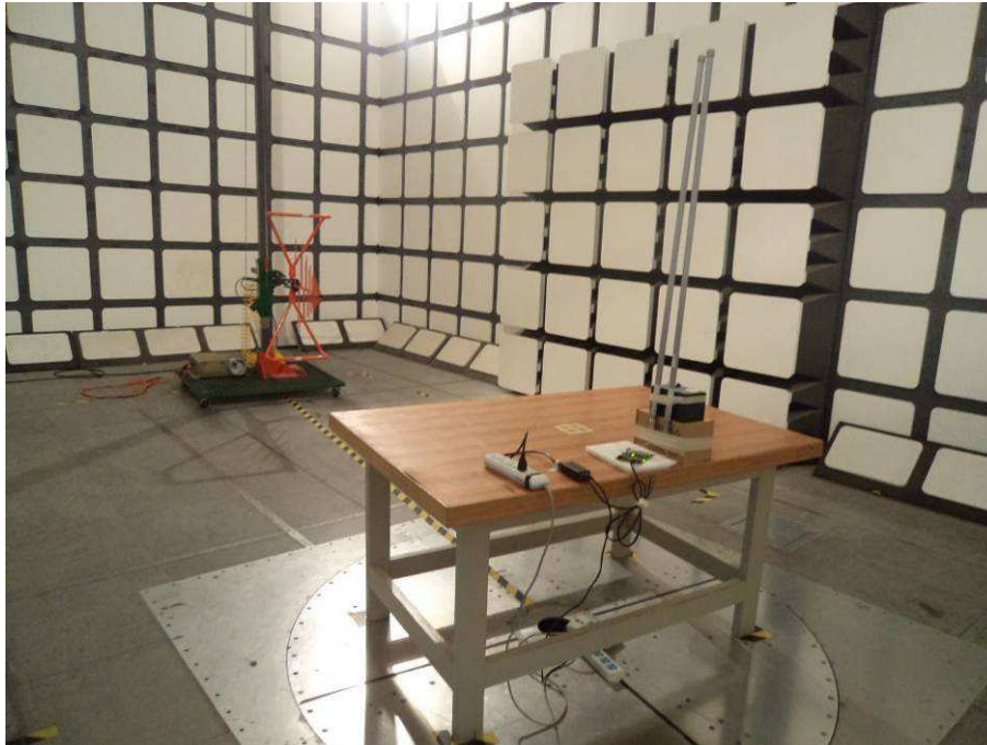
Radiated Emissions View (Below 1 GHz, 12dBi Antenna)
