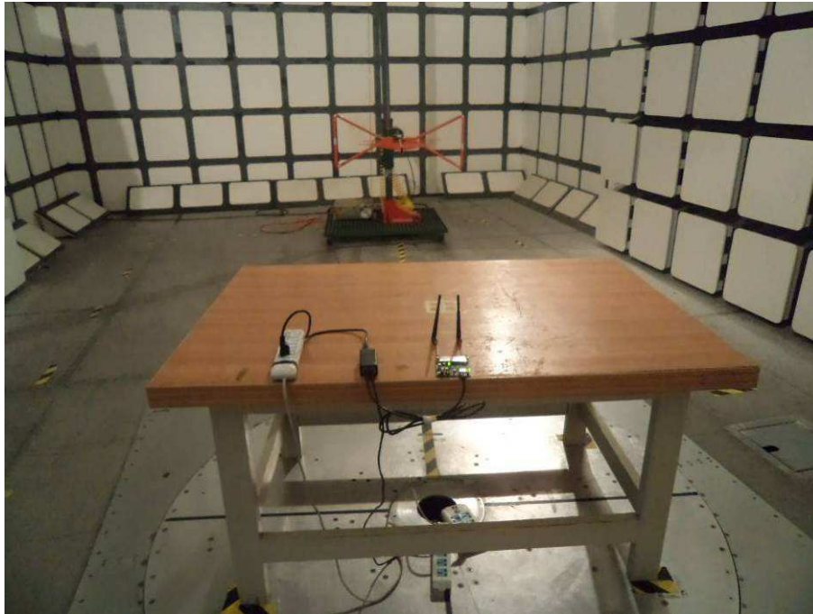
Radiated Emissions View (Below 1 GHz, 3dBi Antenna)
