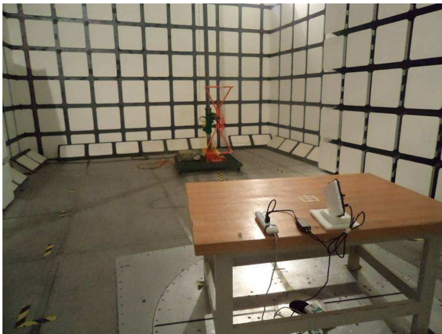
Radiated Emissions View (Below 1 GHz, 14dBi Antenna)
