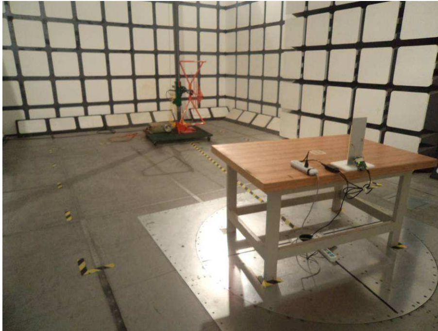
Radiated Emissions View (Below 1 GHz, 16dBi Antenna)
