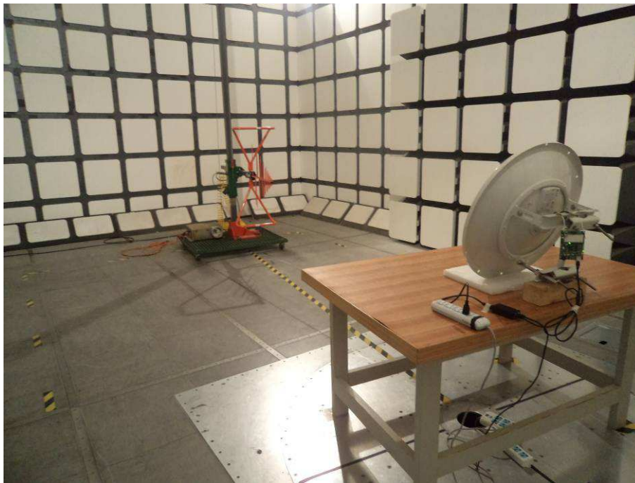
Radiated Emissions View (Below 1 GHz, 24dBi Antenna)
