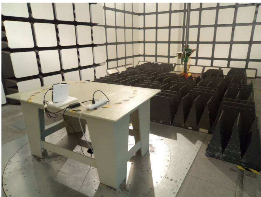
Radiated Emissions View (Above 1 GHz, 14dBi Antenna)
