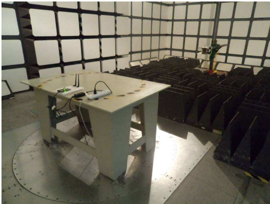
Radiated Emissions View (Above 1 GHz, 3dBi Antenna)
