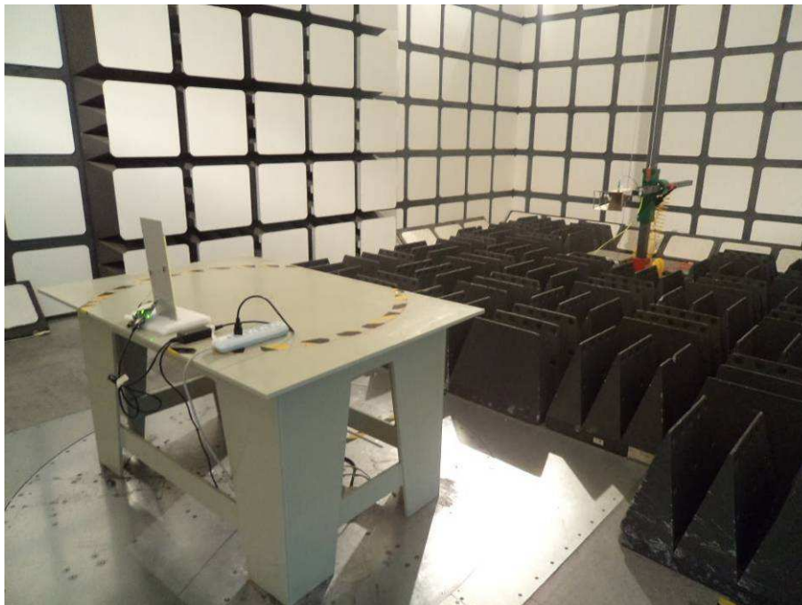
Radiated Emissions View (Above 1 GHz, 16dBi Antenna)
