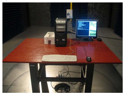
Test Mode: Mode 3: Transmit by 802.11a (7dBi)
