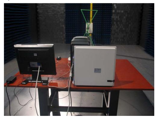
Test Mode: Mode 1: Transmit by 802.11b (19dBi)
