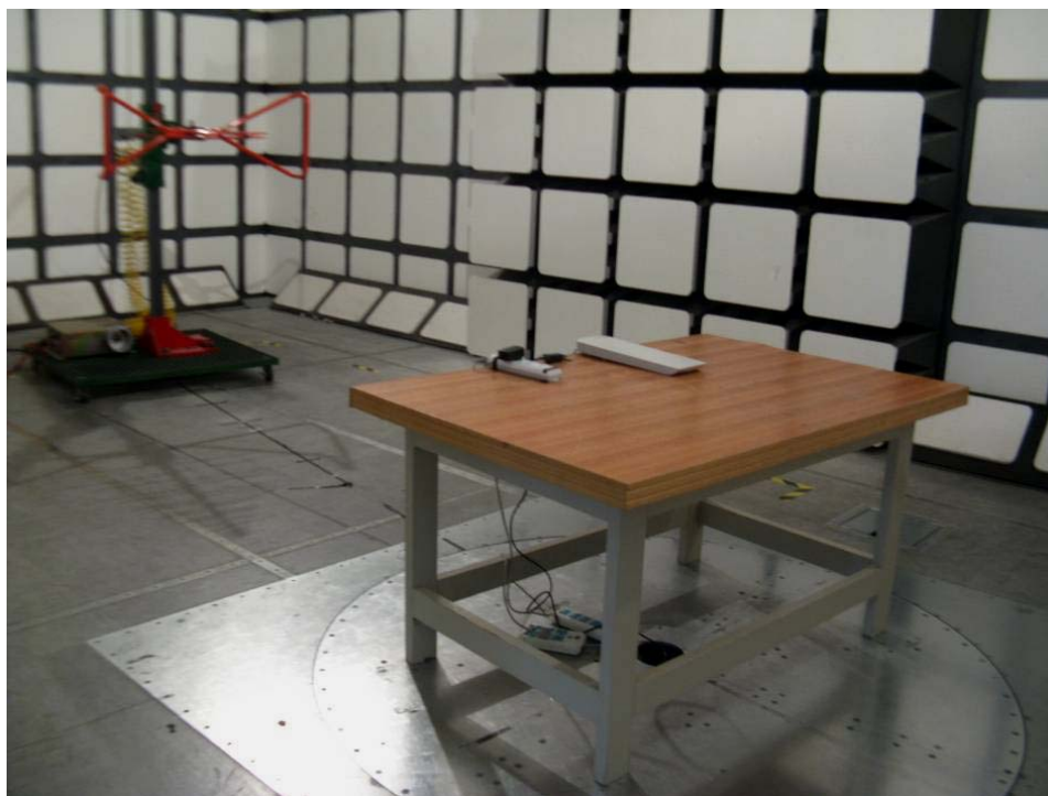
Below 1 GHz: Spurious Radiated Emissions - Rear View
