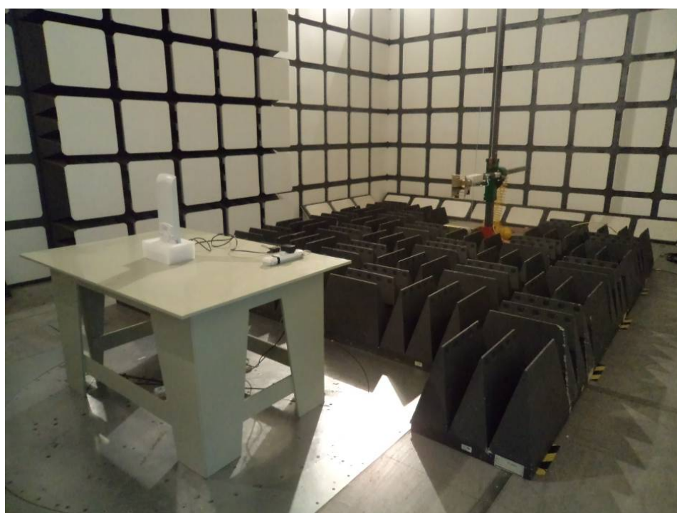
Above 1 GHz: Spurious Radiated Emissions - Rear View
