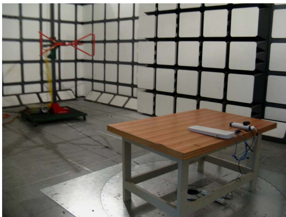
Below 1 GHz: Spurious Radiated Emissions - Rear View
