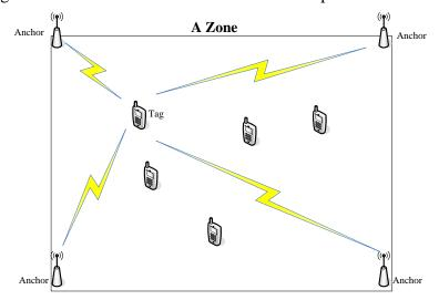
In a minimum system, 4 anchors -3 normal anchors CS5111LP and 1 master anchor CS5113LP- are installed in a zone. However, the more the anchors are installed, the higher the accuracy of the tag position to be obtained.
