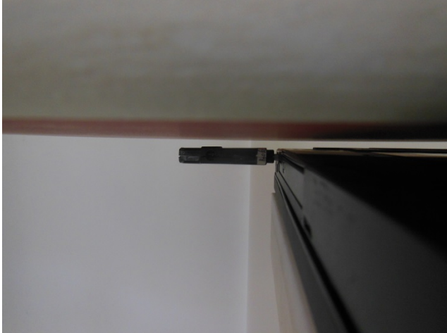
Direct Laptop Plug-in for USB Configuration 1 (Horizontal Up with Phantom 0.5 cm Gap)
