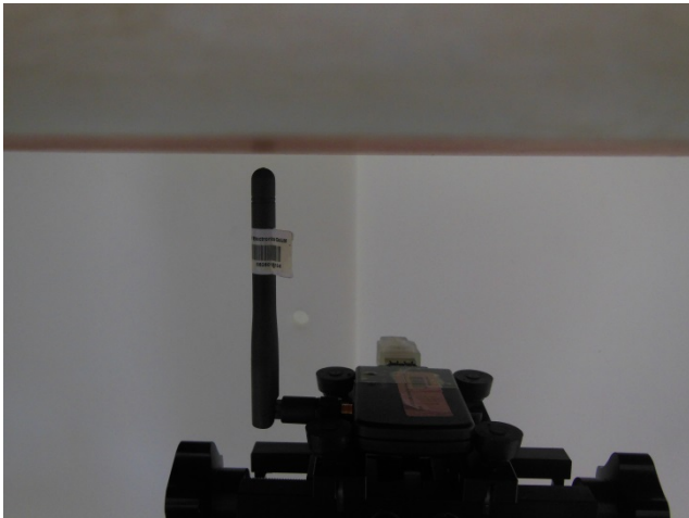
USB Cable Plug-in for USB Configuration 8, (Horizontal Up with Phantom 0.5 cm Gap) with antenna Vertical 90 degree
