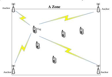
In a minimum system, 4 anchors -3 slave anchors CS5111TD/CS5112TD and 1 master anchor CS5113TD/CS5114TD- are installed in a zone. However, the more the anchors are installed, the higher the accuracy of the tag position to be obtained. The accuracy of positioning is +/-1 meter.
