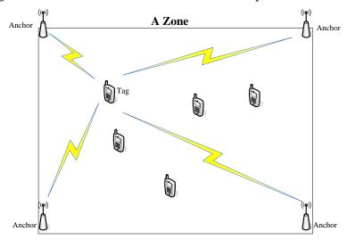
In a minimum system, 4 anchors - 3 normal anchors CS5111LP and 1 master anchor CS5113LP- are installed in a zone. However, the more the anchors are installed, the higher the accuracy of the tag position to be obtained. The accuracy of positioning is +/-1 meter.
