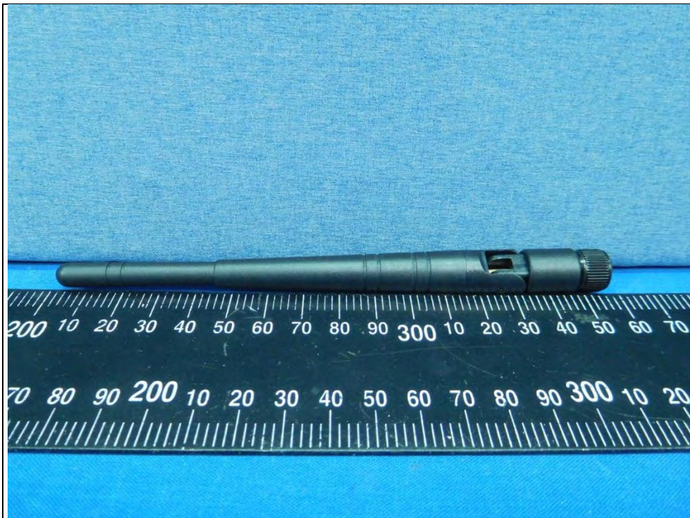
Dipole Antenna (Brand: Taoglas Model: GW.59.3153)
