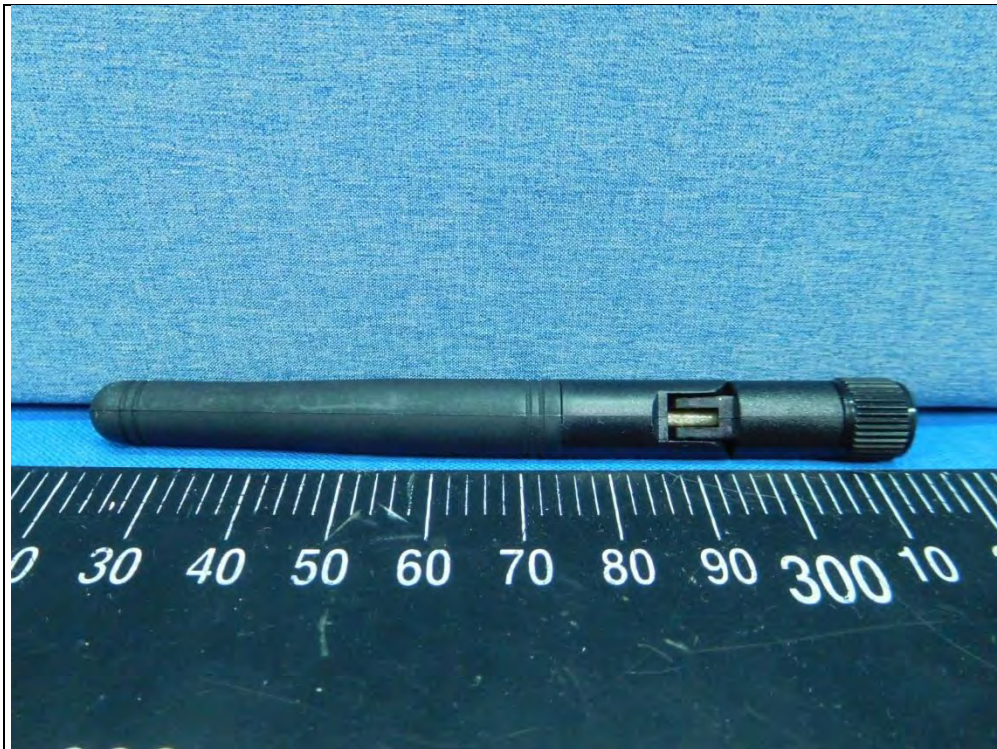
Dipole Antenna (Brand: Laird Model: MAF94051)
