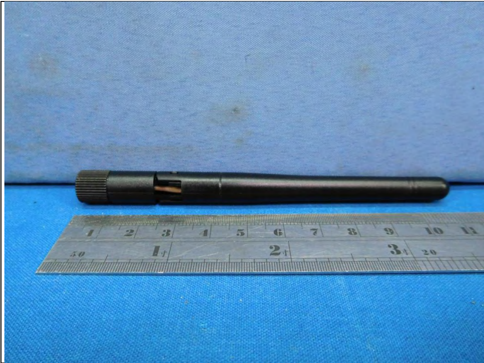
Dipole Antenna (Brand: San Jose Model: UEN-201)
