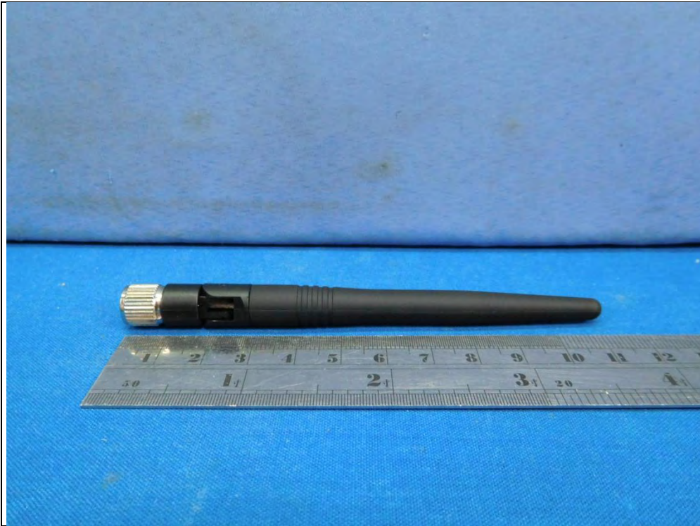
Dipole Antenna (Brand: Bondale Model: G-RA0K10090176-1436B)
