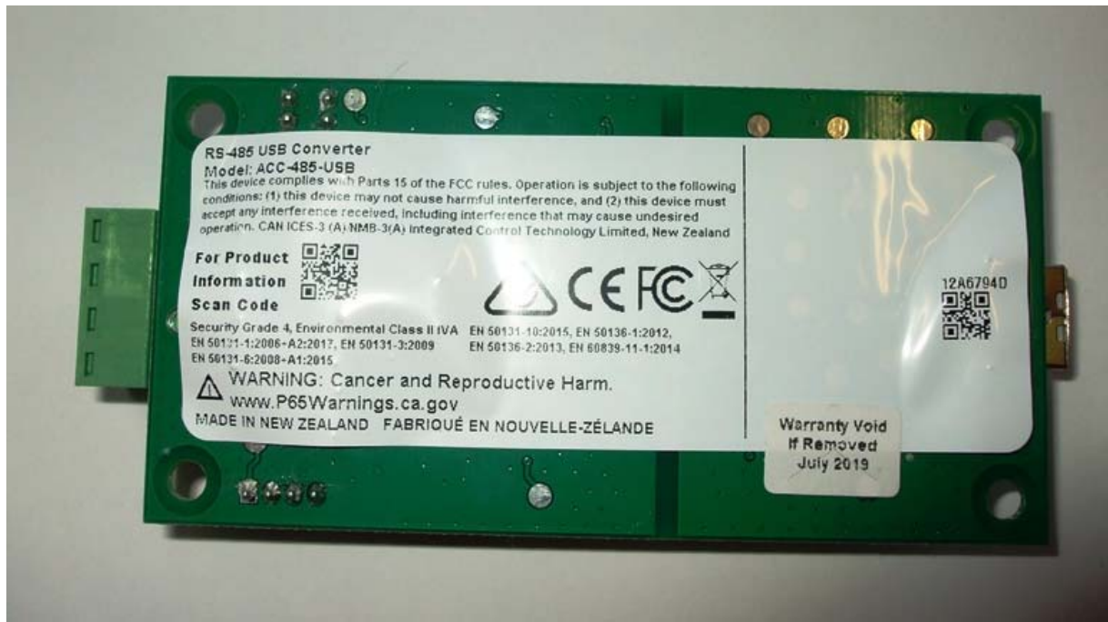
Ancillary: RS-485 to USB to Serial convertor board
