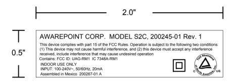
Material: Brady Polyester Thermal Transfer Label P\N: THT-53-423-3 or equivalent Size - 2.0" W x 0.5" H
