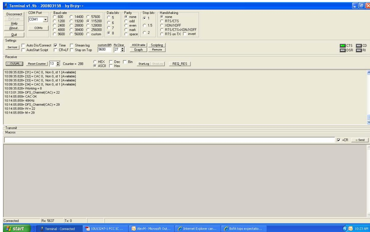
The time stamp at 10:13:01.351 shows the end of the non-occupancy period for the initial channel and the beginning of the subsequent CAC on the initial channel Ch 22 (5560 MHz).
