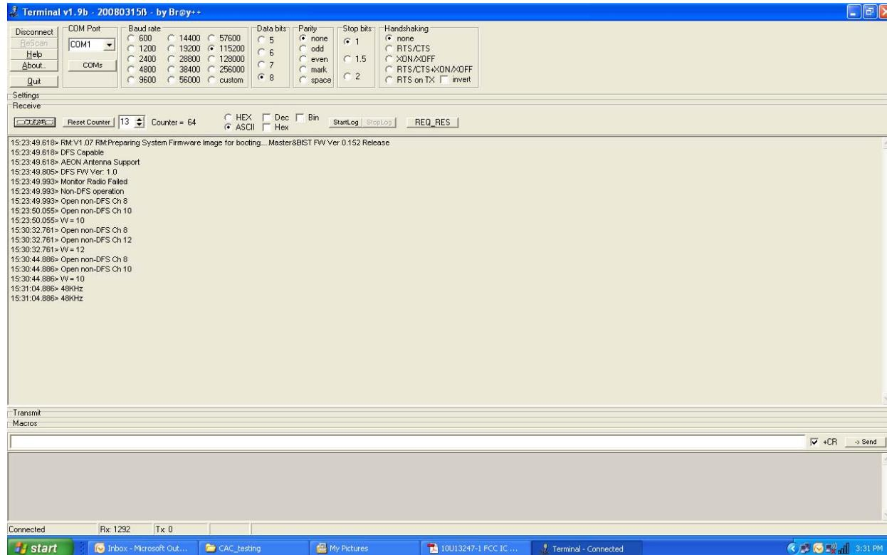
Time stamp 15:23:49.993 shows that the functional check is performed on a non-DFS channel and is not successful. The Working Radio establishes a network on Ch 10 (5200 MHz).
