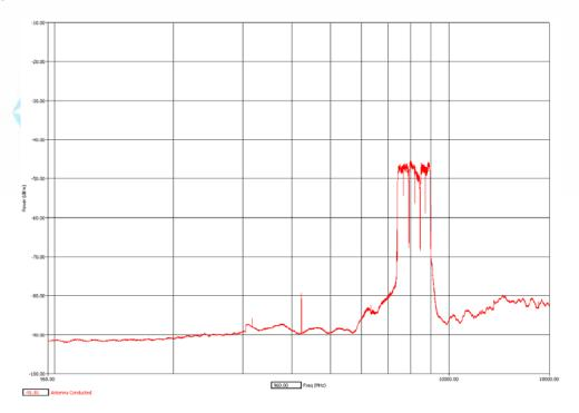
Conducted antenna port measurement made with 1 MHz RBW / 3 MHz VBW Measurement time 1 msec per frequency
