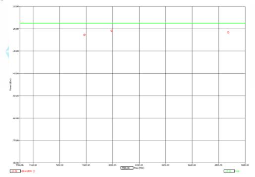
Measurements made with 8 MHz RBW / 8 MHz VBW at 3 meter distance.
