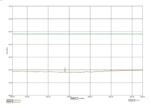
Measurements made with 1 MHz RBW / 3 MHz VBW at 1 meter distance Measurement Time 1 msec per frequency Limit line converted to account for 1 meter measurement distance
