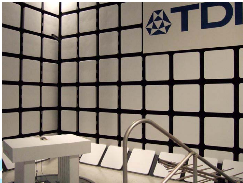
Test Configuration 4: 30 MHz to 960 MHz
