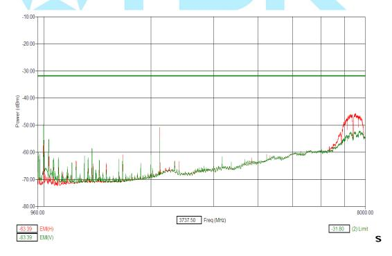
Terminated antenna port measurements made with 1 MHz RBW / 3 MHz VBW at 1 meter distance
