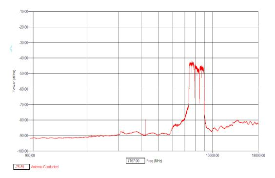
Conducted antenna port measurement made with 1 MHz RBW / 3 MHz VBW Measurement time 1 msec per frequency
