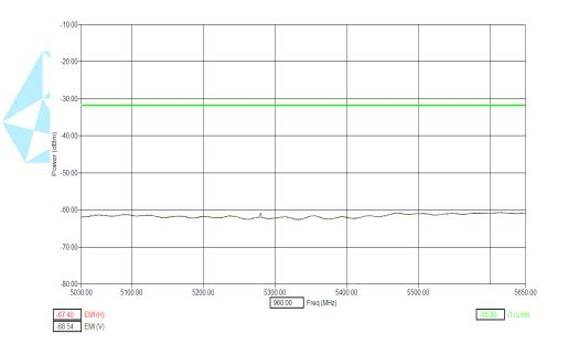
Measurements made with 1 MHz RBW / 3 MHz VBW at 1 meter distance Measurement Time 1 msec per frequency Limit line converted to account for 1 meter measurement distance
