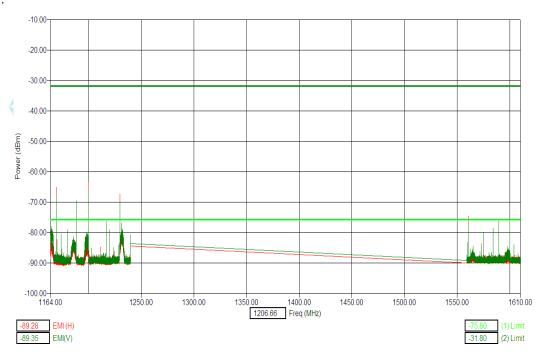
Lower limit line is 47 CFR, Part 15 sub part F
