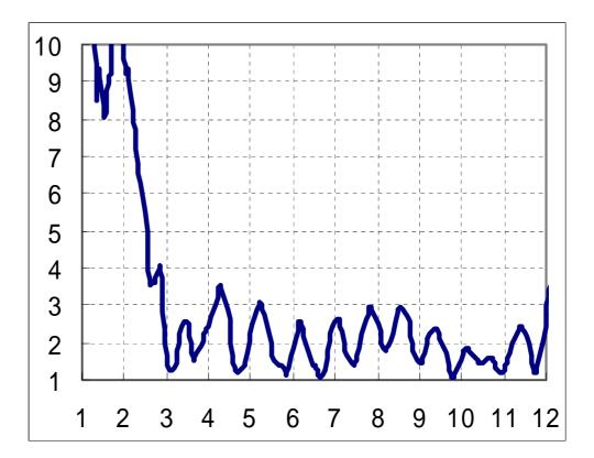
VSWR is 3.6 at maximum in a frequency band from 3.1 to 9.6 GHz.
