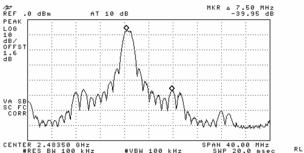
**Band-edges in the restricted band 2483.5 ~ 2500 MHz measurement**
