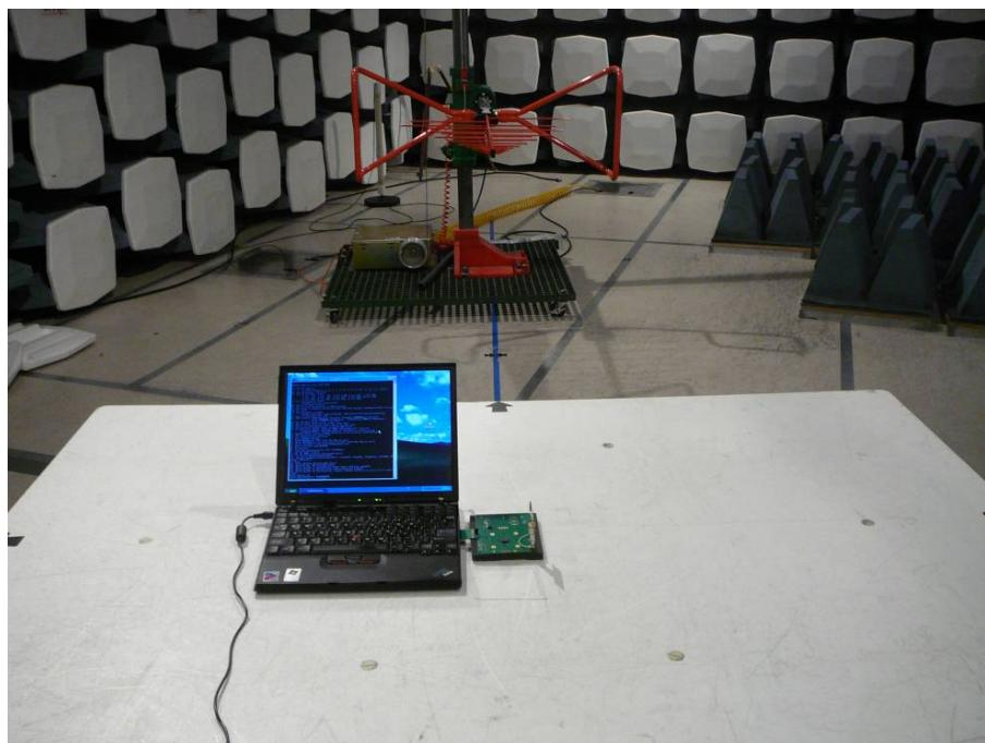
**15.3 Radiated Emission above 1 GHz Front View @ 3 Meter**
