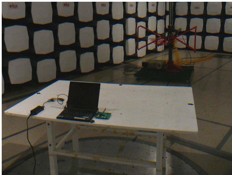
**19.3 Radiated Emission above 1 GHz Front View**
