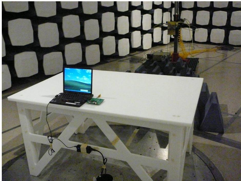
**19.5 AC Line Conducted Emission Front View**
