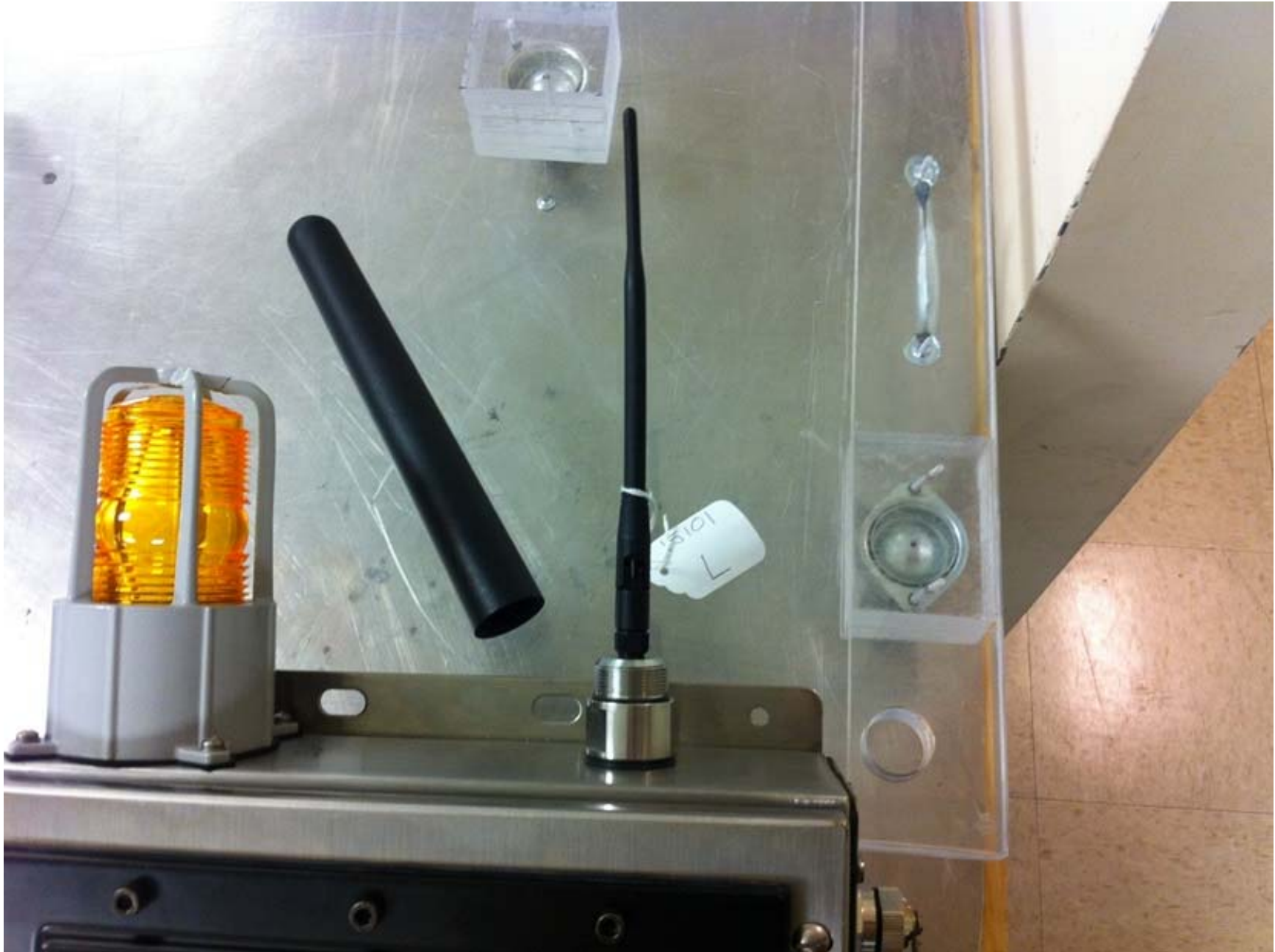
External Antenna As Installed – Protective Cover Removed
