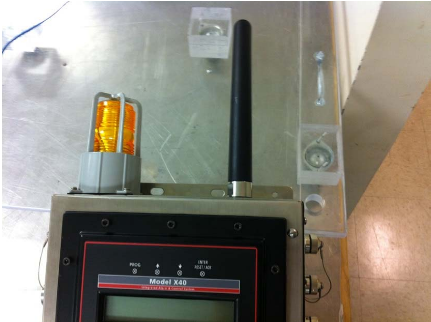
External View of Antenna As Installed – Under Protective Cover
