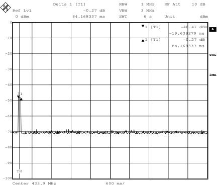
**3. Regulation 15.231 (a2)** A transmitter activated automatically shall cease transmission within 5 seconds after activation.
