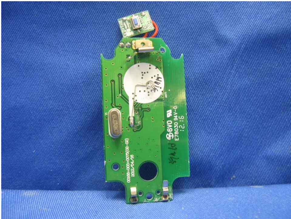
Water Sensor Main PCB comp side (View 2)
