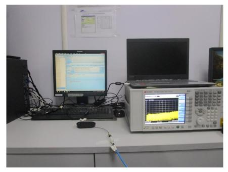
1.2 Fundamental Emission & Radiated Emission (below 1GHz) Test Setup
