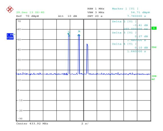
The plot shows the fundamental emission when modulated.
