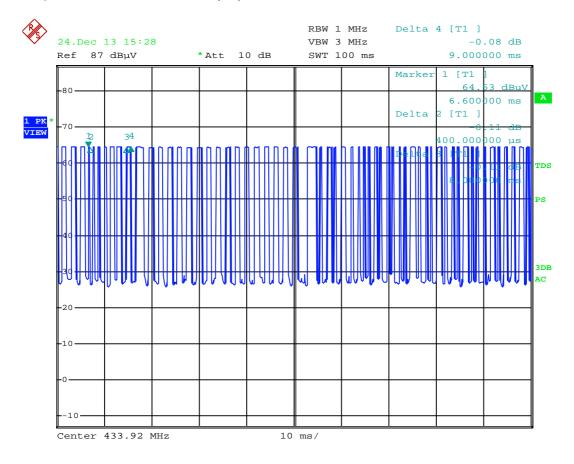
A plot of the worst-case duty cycle as detected in this manner is shown below.
