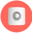
Motion Sensor On a shelf or adhere 4–5 ft high in a corner
