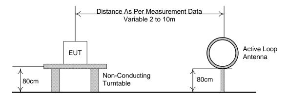
Open Area Test Site – Flat Level Area – Asphalt Surface – Clear Of Obstacles
