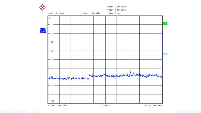
**Notes:** The measurement range from 30 - 40 GHz has been transposed by a mixer of 20 GHz to the analyzer range from 10 - 20 GHz.
