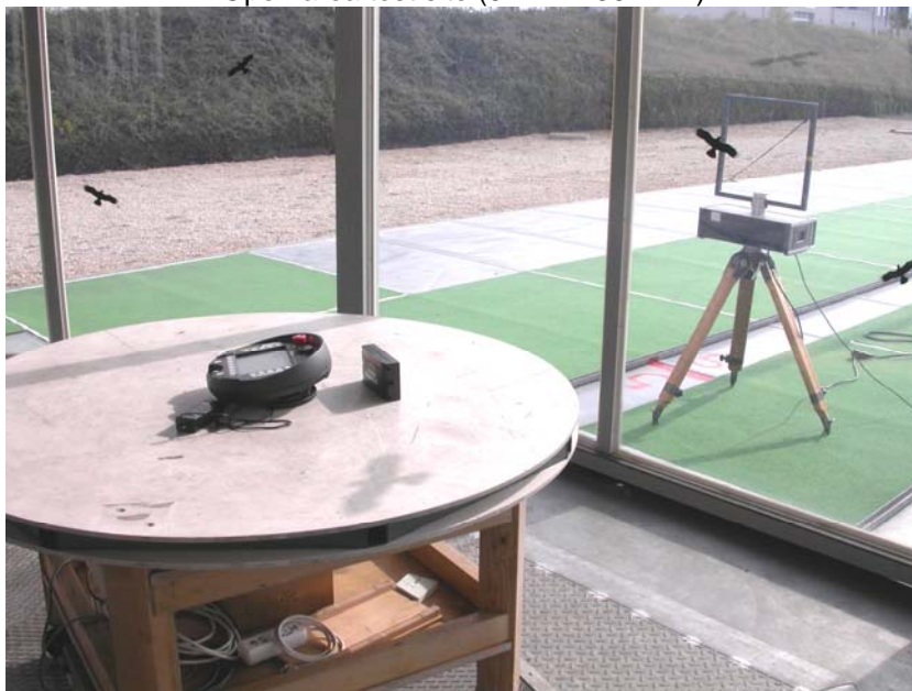
Open area test site (9 kHz – 30 MHz)
