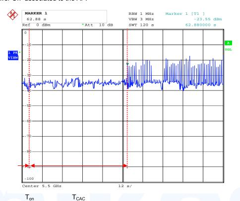
$T_{on}$  = 2.88 s (time for boot and system setup))  $T_{CAC}$  = 60 s (Channel availability check)
