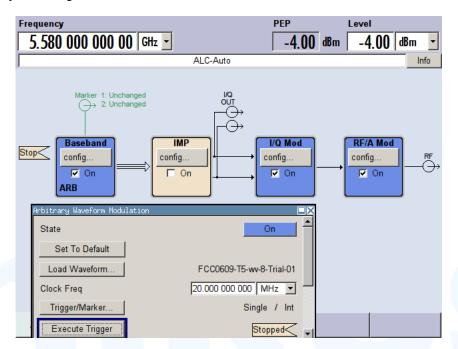
The appropriate radar test pattern is generated by an R&S SMBV100A (Vector SG with one ARB). The K6 sequencer software has been used for creating complex waveforms to generate the puls and burst sequence.
