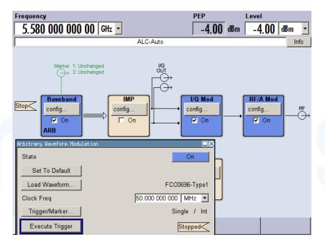
The appropriate radar test pattern is generated by an R&S SMBV100A (Vector SG with one ARB). The K6 sequencer software has been used for creating complex waveforms to generate the puls and burst sequence.
