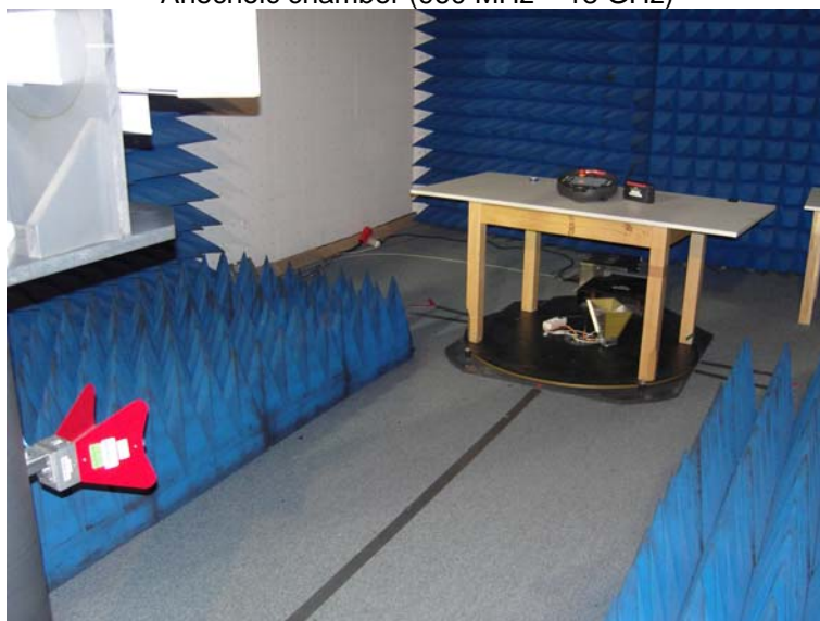
Anechoic chamber (960 MHz – 18 GHz)
