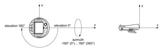
The figure below shows the range of the transmitter based on angle.
