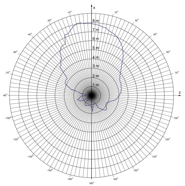
The following figure shows the transponder range depending on the angular displacement to the main count direction in the z direction:
