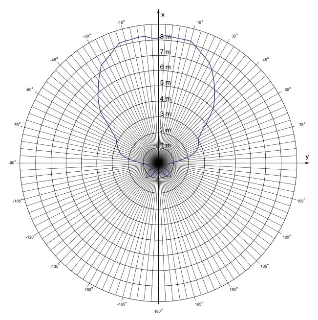
The figure below shows the range of the transmitter based on angle.
