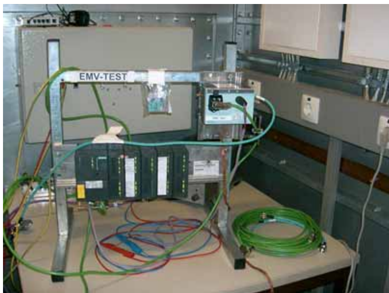
Photo 11: Test setup for radiated RF-emission (Periphery outside chamber)
