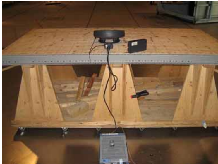
Photo 3: Test setup for AC powerline conducted emission (rear side)
