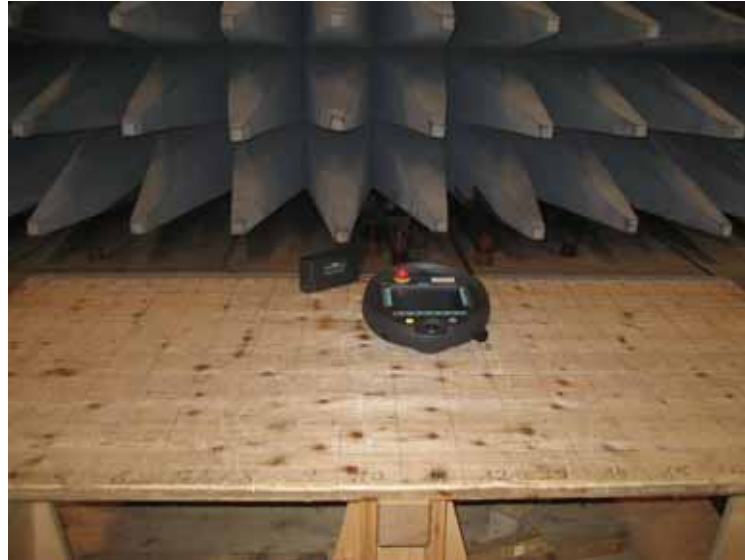
Photo 1: Test setup for AC powerline conducted emission (front side)
