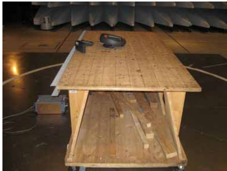
Photo 2: Test setup for AC powerline conducted emission (left side)
