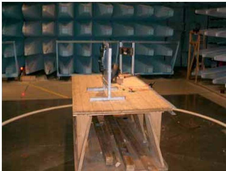
Photo 7: Test setup for radiated RF-emission (right side)
