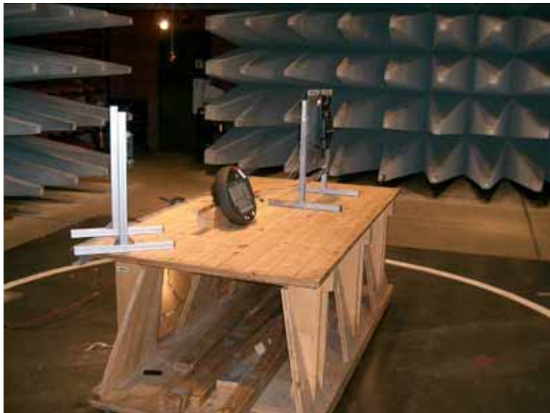
Photo 9: Test setup for radiated RF-emission (left side)
