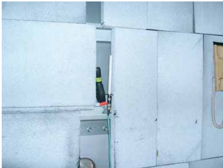
Photo 10: Test setup for radiated RF-emission (Antenna for WLAN connection)
