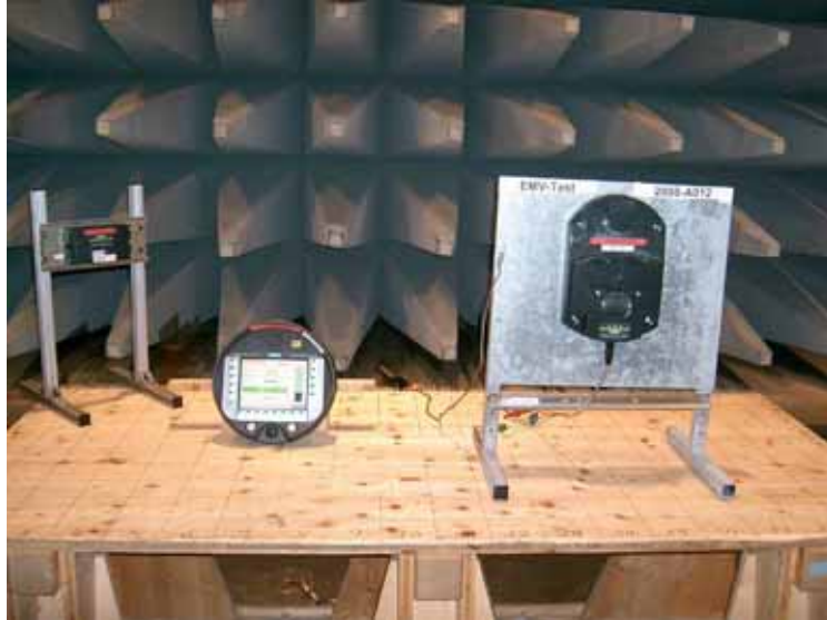
Photo 6: Test setup for radiated RF-emission (front side; transponder left side, Mobile Panel in the middle and loading cradle on right side)
