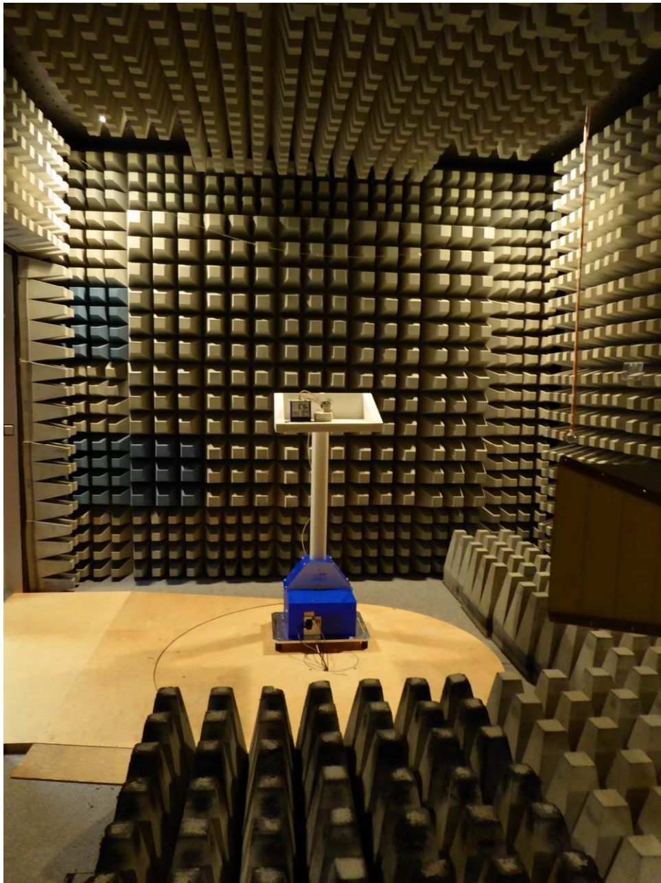
160308_04: Test setup - Radiated emission anechoic chamber, cabinet emissions
