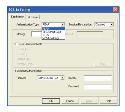
The IEEE 802.1X specification describes a protocol that can be used for authenticating both clients and servers on a network. The authentication algorithms and methods are those provided by the Extensible Authentication Protocol (EAP), a method of authentication that has been in use for a number of years on networks that provide Point-to-Point Protocol (PPP) support as many internet service providers and enterprises do.
