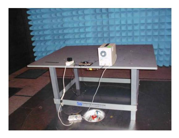
1GHz – 25GHz, transferring audio signal mode from an audio generator
