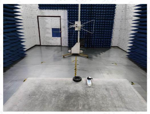
RADIATED EMISSION TEST SETUP ABOVE 1GHz
