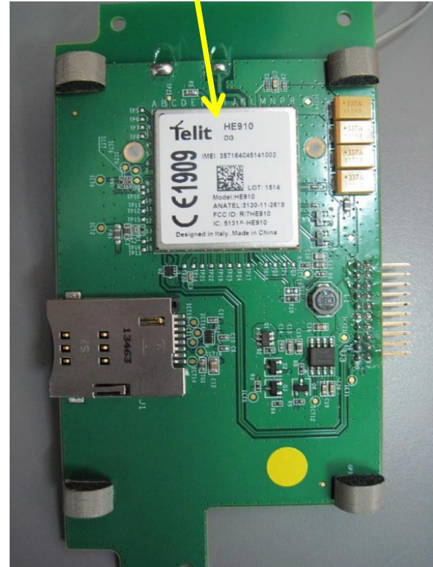
Tellit modem with FCC-ID, in the bottom side
