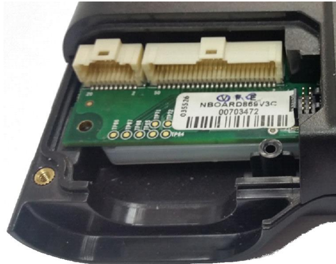
Figure 8: SmartHub Underdash OBC Interface connectors
