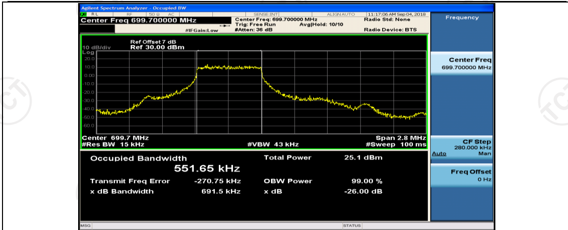
(Channel Bandwidth: 1.4 MHz)_LCH_QPSK_3RB#2
