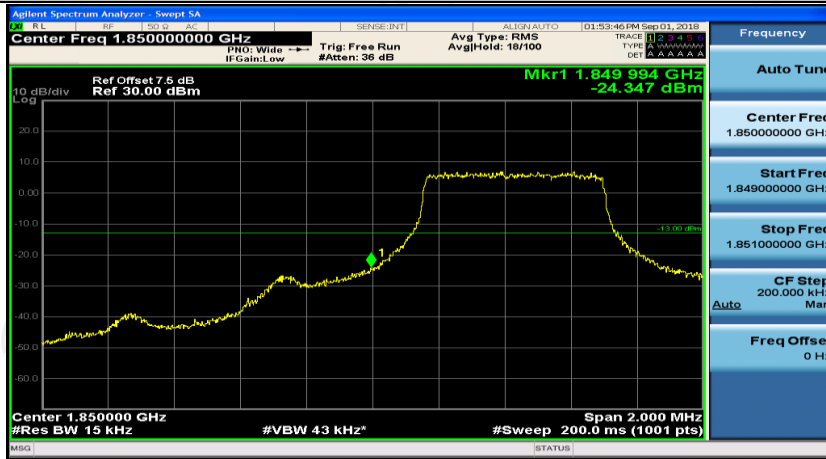
(Channel Bandwidth: 1.4 MHz)_LCH_QPSK_3RB#2
