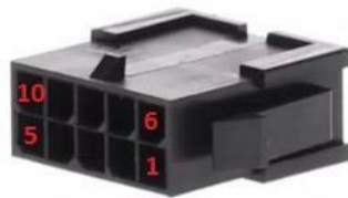
Figure 14: Molex 10-Pin Male Connector
