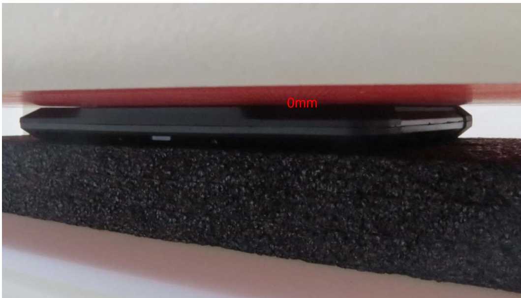
Picture 2: Front Side, the distance from handset to the bottom of the Phantom is 0mm
