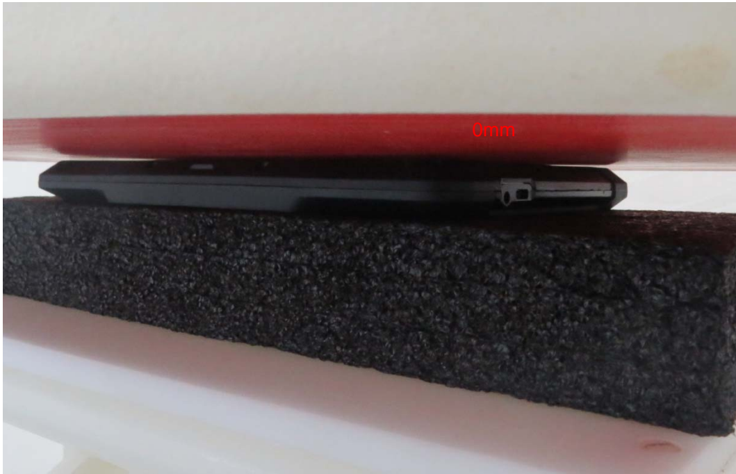
Picture 1: Back Side, the distance from handset to the bottom of the Phantom is 0mm
