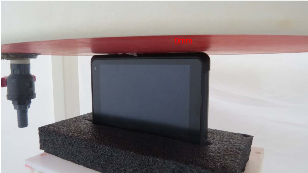
Picture 5: Top Side, the distance from handset to the bottom of the Phantom is 0mm
